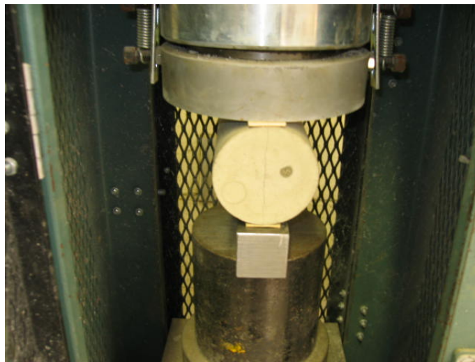
Figure 3.2 Split Tensile Strength Test (ASTM C596)
