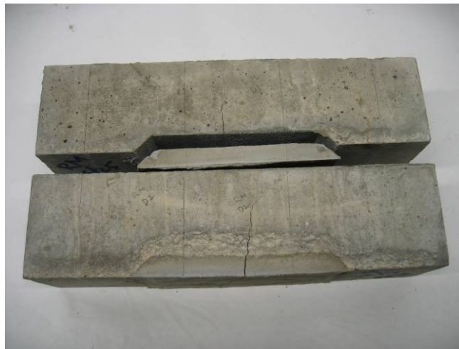
(b) Failure due to de-lamination
