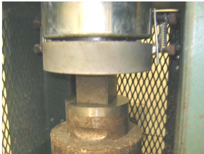
Figure 3.1 Compressive Strength Test (ASTM C109)
