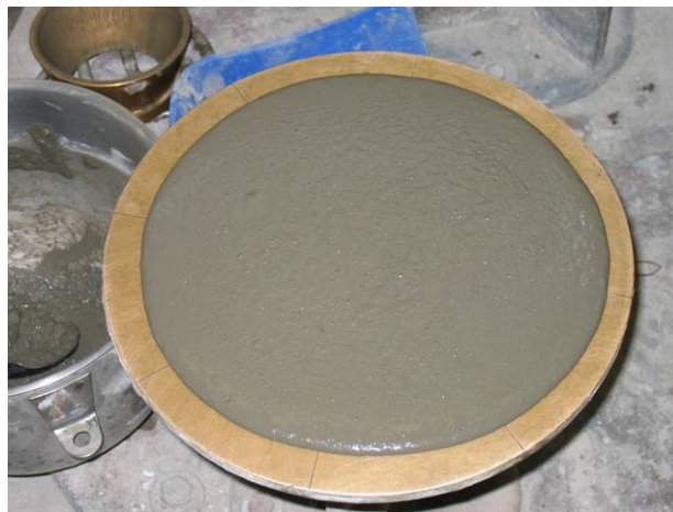
Figure 4.1 Flow of Repair Material (Note: Fig. 4.1 shows a flow of 113%)
