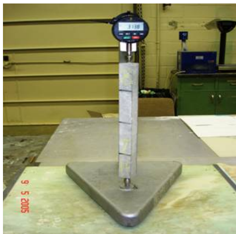
Figure 3.3 Comparator Readings for Length-Change Measurement
