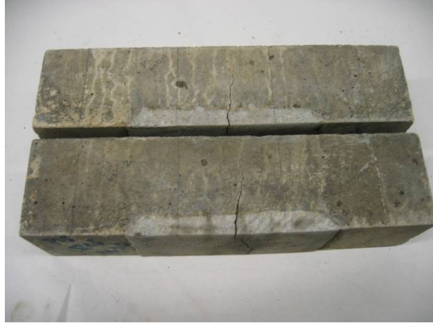
(a) Failure at the center
