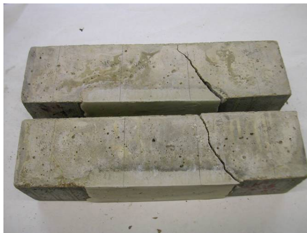
(c) Failure at the edge of repair
