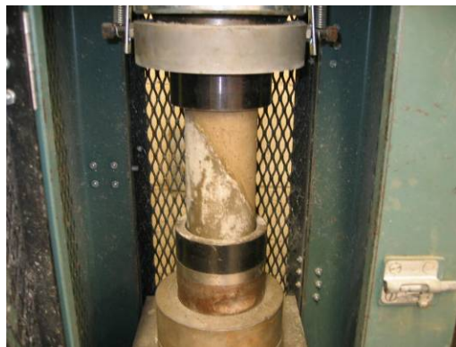
Figure 3.5 Slant Shear Test (ASTM C882)
