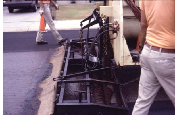
Figure 8: Slurry Seal Box with Augers (8)
