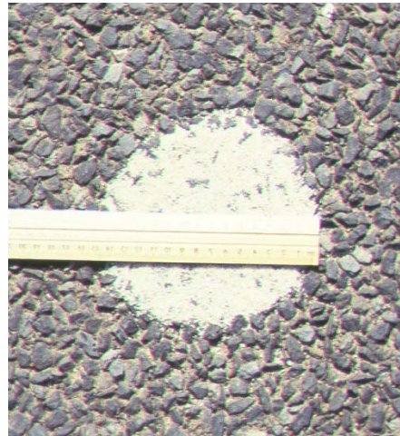
b) Sand Patch Test
