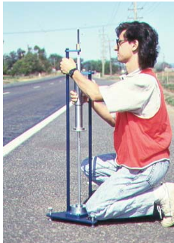
a) Ball Penetrometer Test
