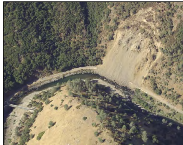
Aerial view of landslide onto Highway 140 and the newly constructed detour bridge
