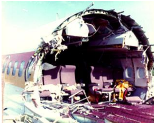
Figure 5: Front view of Damaged Aloha Airline Flight 243 fuselage
