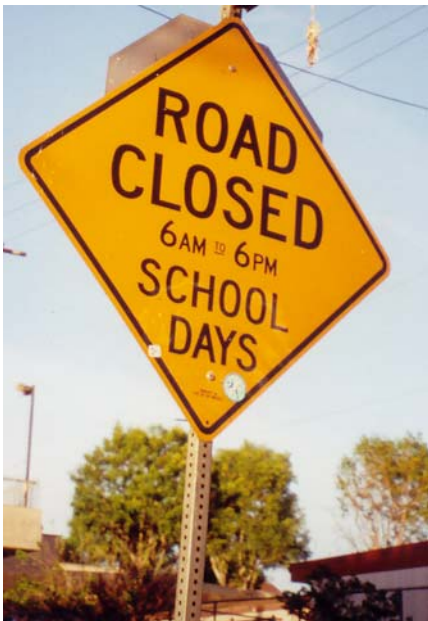
Figure 7-44. Example of Sign Used to Close Road During School Hours.
