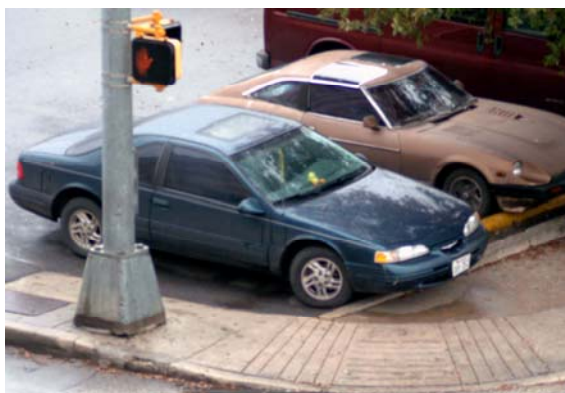
Figure 7-10. Parked Vehicle and Signal Pole Block Pedestrian Travel Near Northeast Corner of Intersection.
