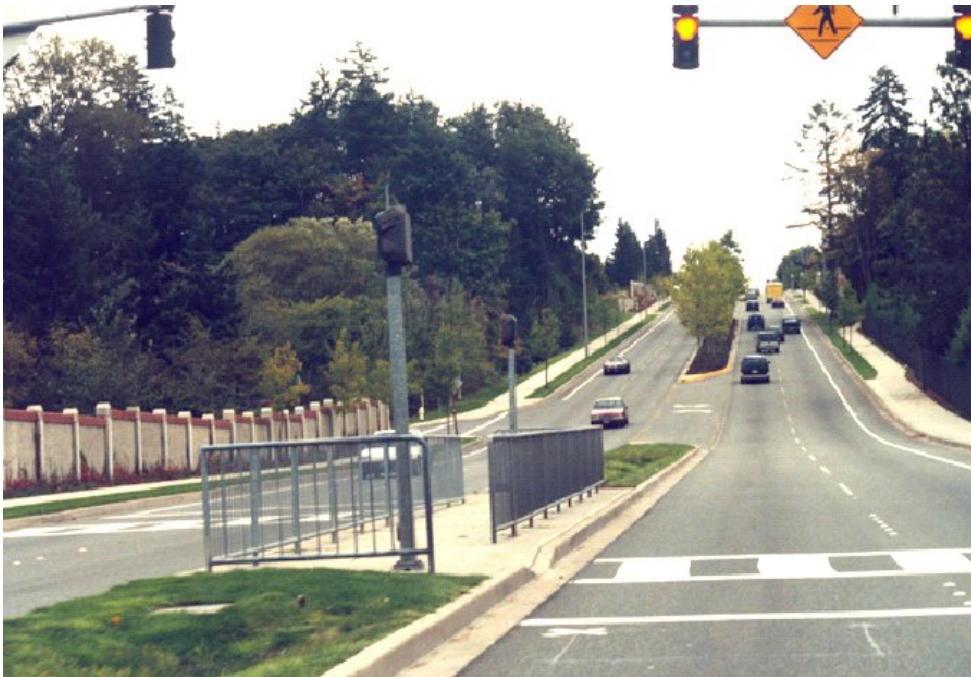
Figure 7-36. Split Midblock Signal Treatment in Bellevue.
