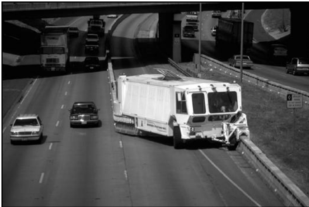
Figure 6-24. Movable Barrier Used in Dallas. (9)
