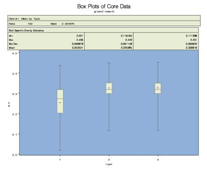
Figure 4.18 Bulk Specific Gravity Data by Method of Fine-Graded NMAS 5 Cores
