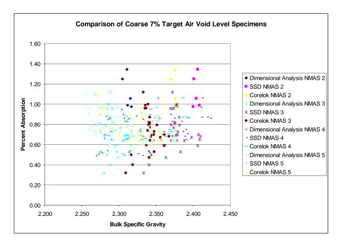
Figure 4.6 Comparison Between Bulk Specific Gravity and Percent Absorption for Coarsegraded 7% Target Air Void Level Specimens
