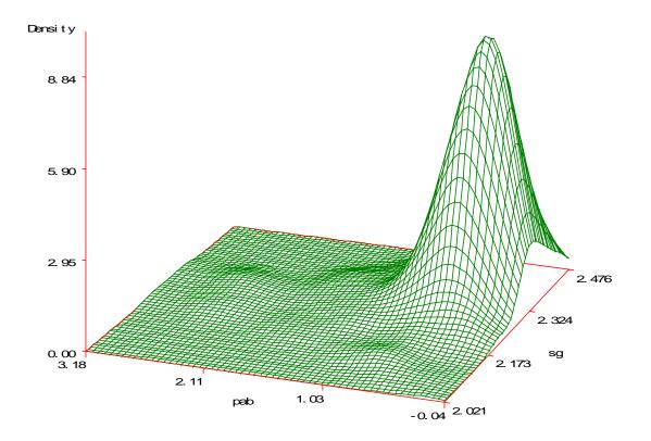
Figure 4.21 Density Plot Relating Percent Absorption to Bulk Specific Gravity
