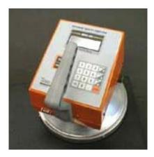
Figure 2.2 Pavement Quality Indicator<sup>TM</sup>
