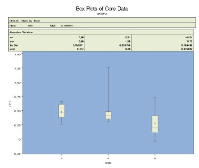
Figure 4.11 Percent Absorption Data by NMAS for Fine-Graded Cores
