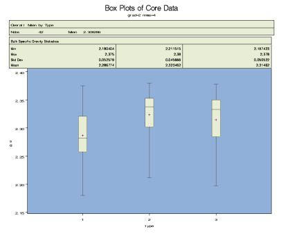
Figure 4.17 Bulk Specific Gravity Data by Method of Fine-Graded NMAS 4 Cores
