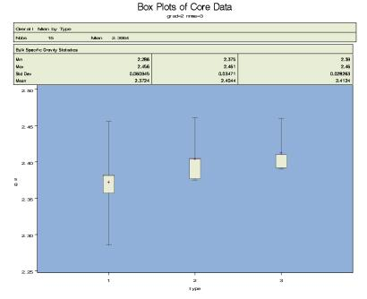
Figure 4.16 Bulk Specific Gravity Data by Method of Fine-Graded NMAS 3 Cores
