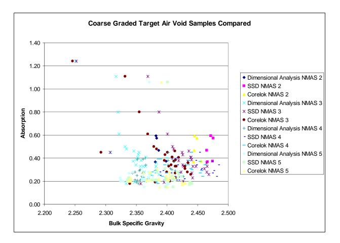
Figure 4.5 Comparison Between Bulk Specific Gravity and Percent Absorption for Coarsegraded 4% Target Air Void Level Specimens
