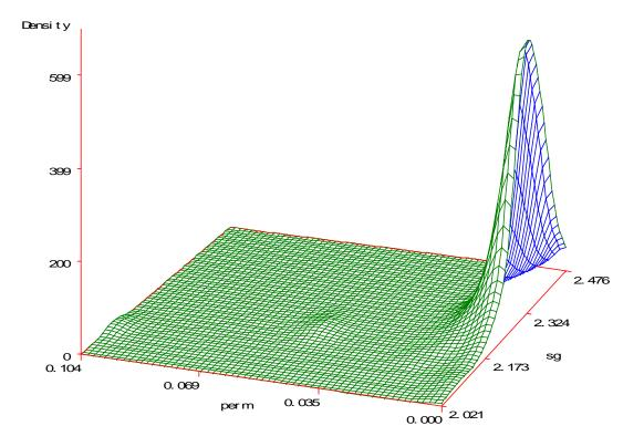
Figure 4.20 Density Plot Relating Permeability to Bulk Specific Gravity
