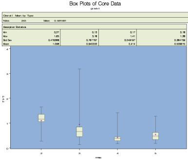
Figure 4.10 Percent Absorption Data by NMAS for Coarse-Graded Cores
