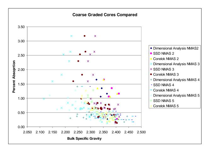
Figure 4.4 Comparison Between Bulk Specific Gravity and Percent Absorption for Coarsegraded Cores
