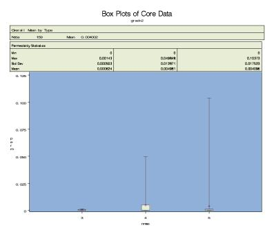
Figure 4.9 Permeability Data by NMAS for Fine-Graded Cores
