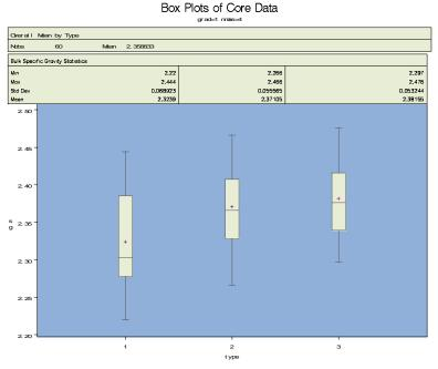
Figure 4.14 Bulk Specific Gravity Data by Method of Coarse-Graded NMAS 4 Cores
