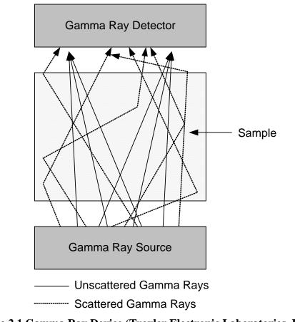
Figure 2.1 Gamma Ray Device (Troxler Electronic Laboratories, Inc.)
