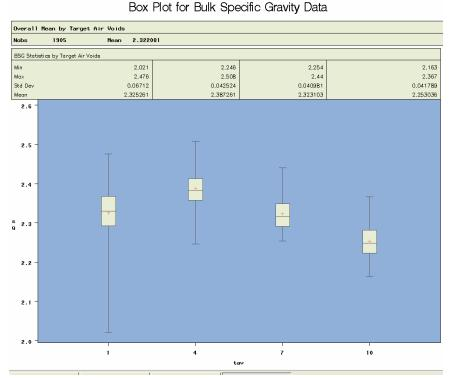
Figure 4.3 Box Plot of All Bulk Specific Gravity Values by Target Air Void Level
