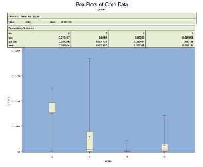
Figure 4.8 Permeability Data by NMAS for Coarse-Graded Cores
