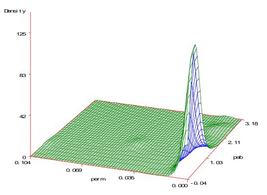
Figure 4.19 Density Plot Relating Permeability to Percent Absorption
