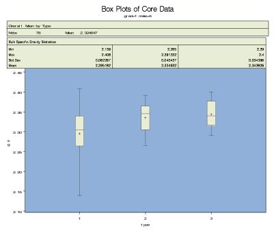
Figure 4.15 Bulk Specific Gravity Data by Method of Coarse-Graded NMAS 5 Cores
