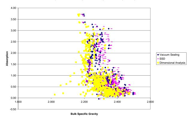
Comparison of Bulk Specific Gravity Methods By Absorption
