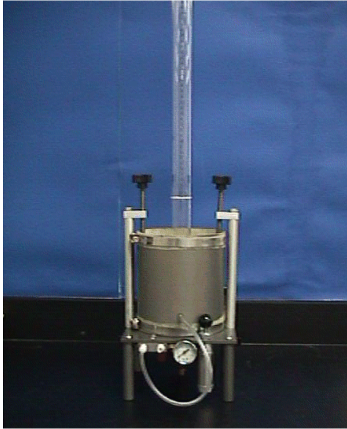
Figure 7– Water Permeability Laboratory Testing Apparatus
