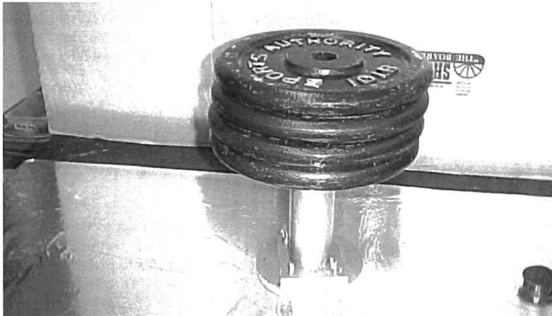
Figure 6.13 - Loading Arrangement for Simple Pull-Off Test
