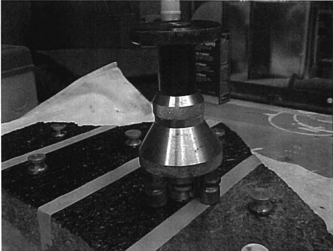
Figure 3.5 - Test Performed using ELCOMETER106
