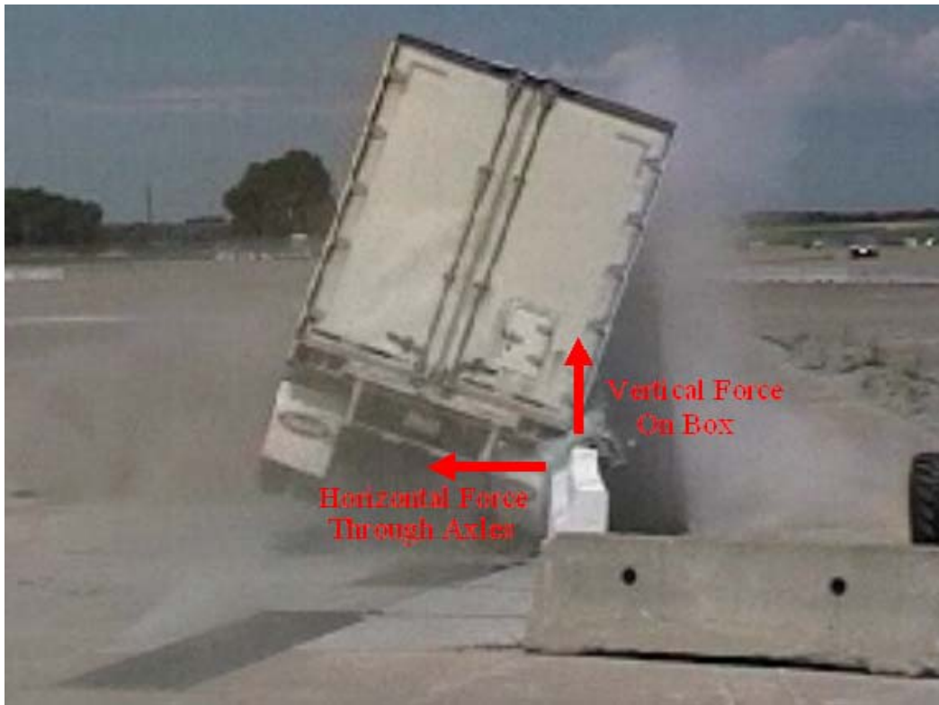
Figure 33. Forces Acting on a Tractor Trailer during Impact.
