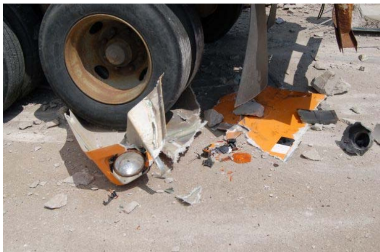
Figure 92. Damage to Rear of Vehicle, Test TL5CMB-2
