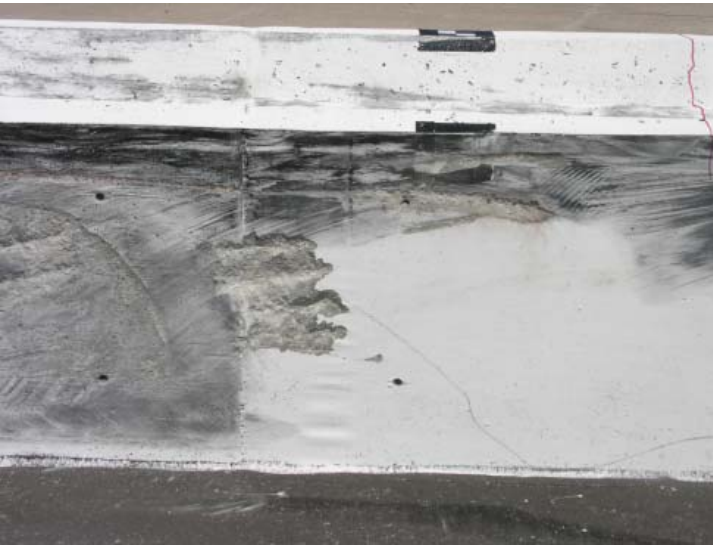
Figure 80. Barrier Damage, Gouges 9.1 - 11.0 m (30 - 36 ft) from Upstream End, Test TL5CMB-2
