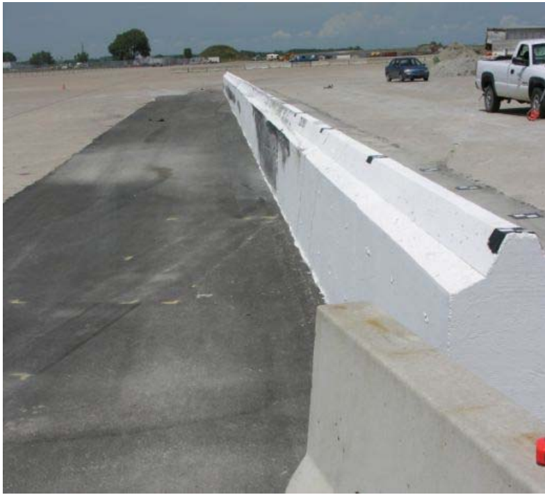
Figure 72. Vehicle Final Position and Trajectory Marks, Test TL5CMB-2
