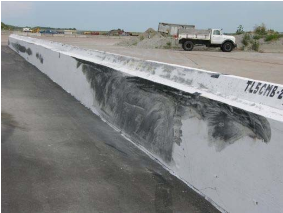
Figure 73. Barrier Damage, Test TL5CMB-2
