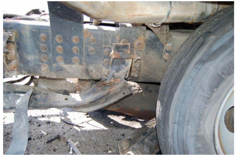
Figure 88. Right Side Tractor Damage, Test TL5CMB-2
