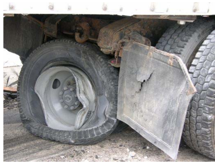
Figure 90. Vehicle Damage to Front Tandems, Test TL5CMB-2
