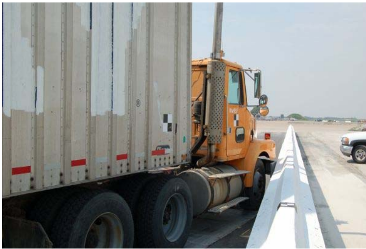
Figure 71. Impact Location, Test TL5CMB-2
