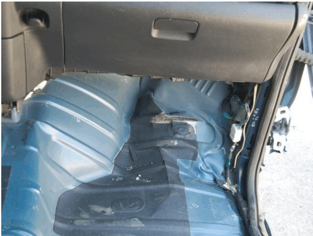
Figure 68. Occupant Compartment Damage, Test No. TCBT-2
