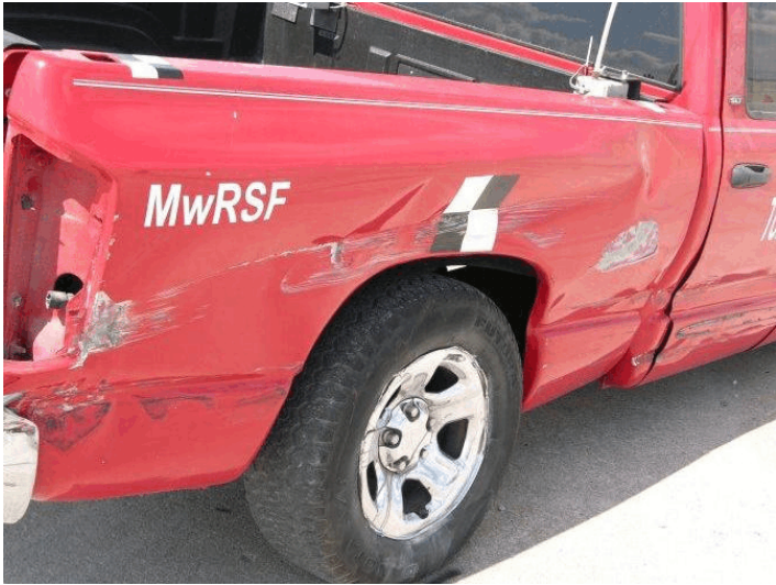
Figure 52. Vehicle Damage, Test No. TCBT-1
