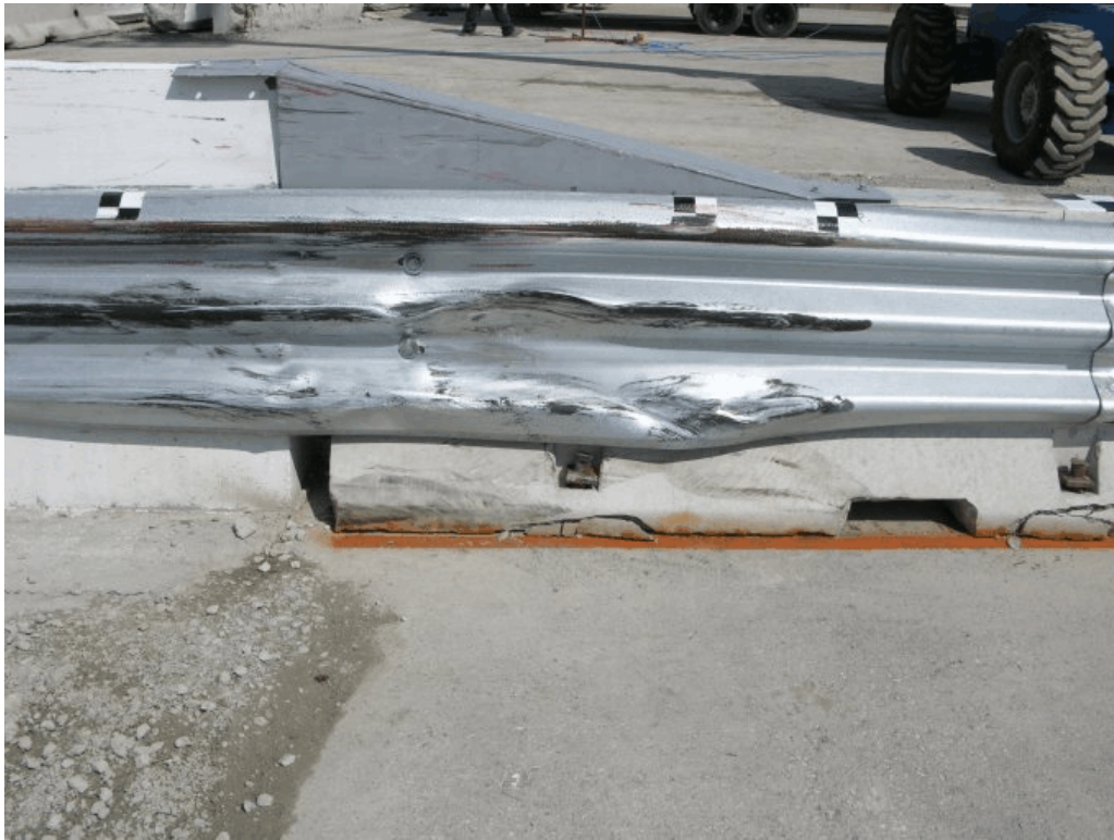
Figure 46. System Damage, Test No. TCBT-1
