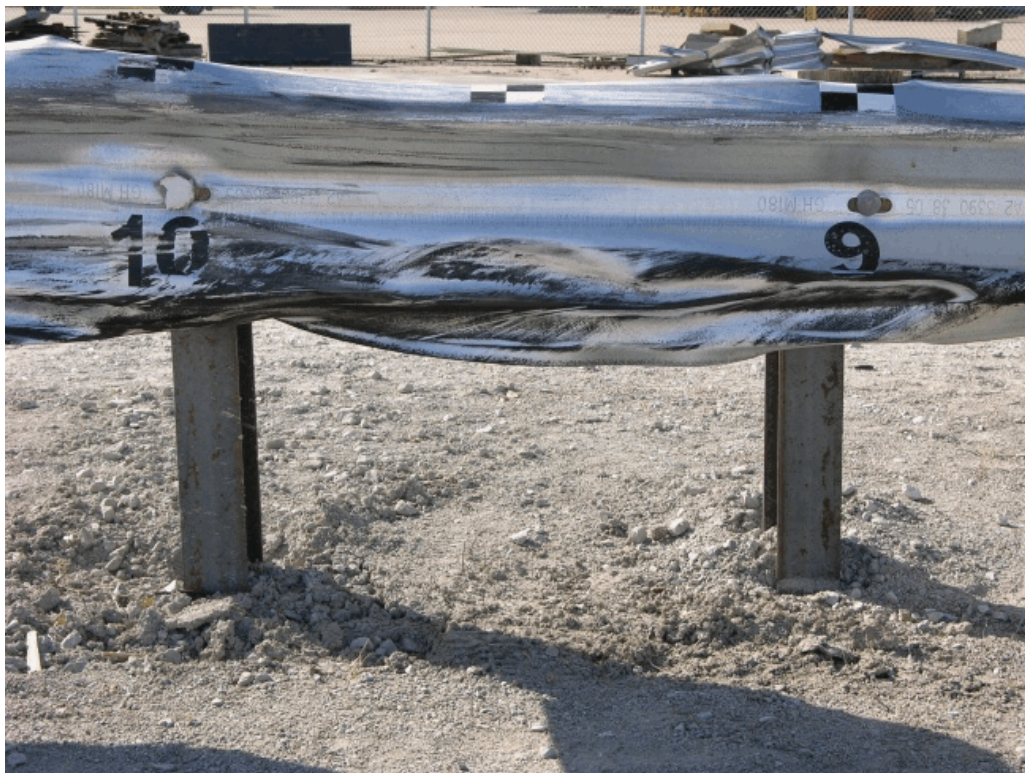
Figure 109. Post Nos. 8 through 10 Damage, Test MWT-5
