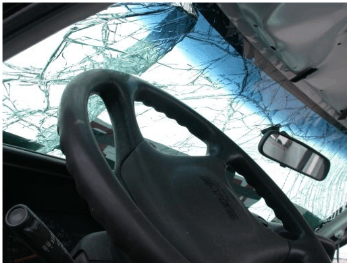
Figure 49. Occupant Compartment and Windshield Damage, Test MWT-3
