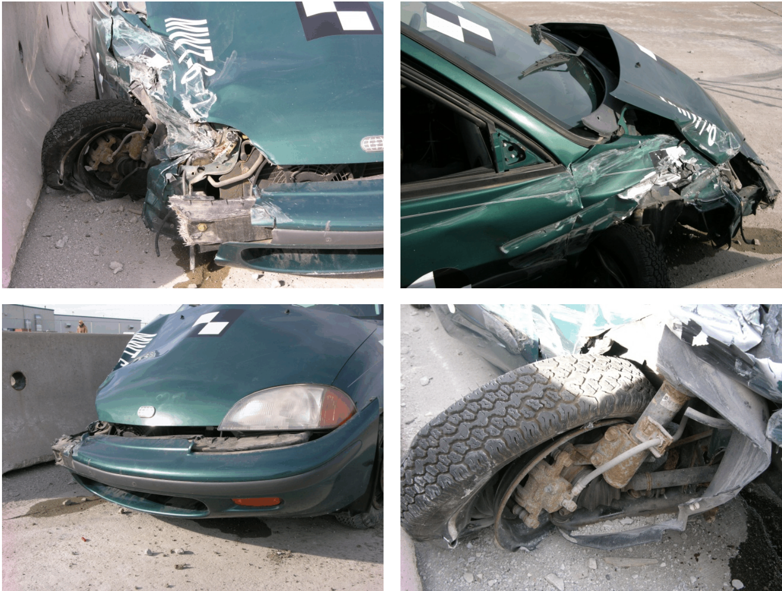
Figure 130. Vehicle Damage, Test MWT-6
