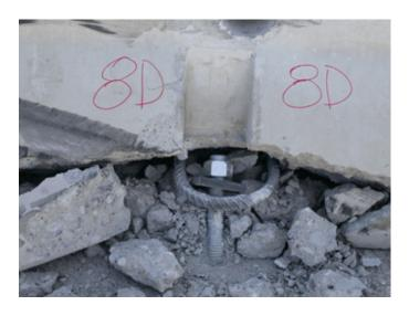
Figure 28. Barrier No. 8 Tie-Down Anchor Damage, Test KTB-1
