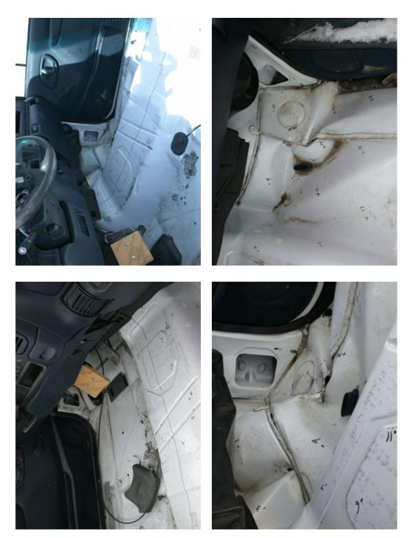
Figure 34. Occupant Compartment Damage, Test KTB-1
