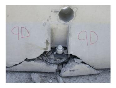
Figure 29. Barrier No. 9 Tie-Down Anchor Damage, Test KTB-1
