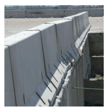
Figure 25. System Damage, Test KTB-1
