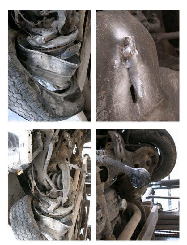
Figure 33. Vehicle Undercarriage Damage, Test KTB-1
