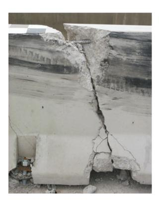
Figure 27. Barrier Nos. 8 and 9 Concrete Damage, Test KTB-1
