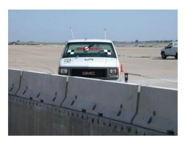
Figure 22. Impact Location, Test KTB-1
