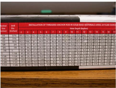
Figure C-2. Epoxy Specifications
