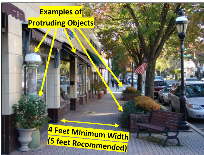
Figure 21: PAR Clear Width Excluding Protruding Objects
