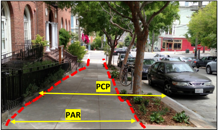
Figure 1: PAR within Pedestrian Circulation Path
