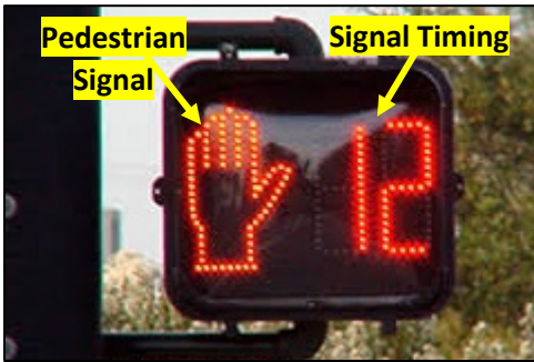
Figure 78: Pedestrian Signals Combined with Pedestrian Signal Timing
