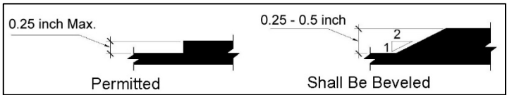
Figure 17: Vertical Surface Discontinuity
