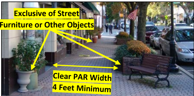
Figure 5: PAR Width and Street Furniture
