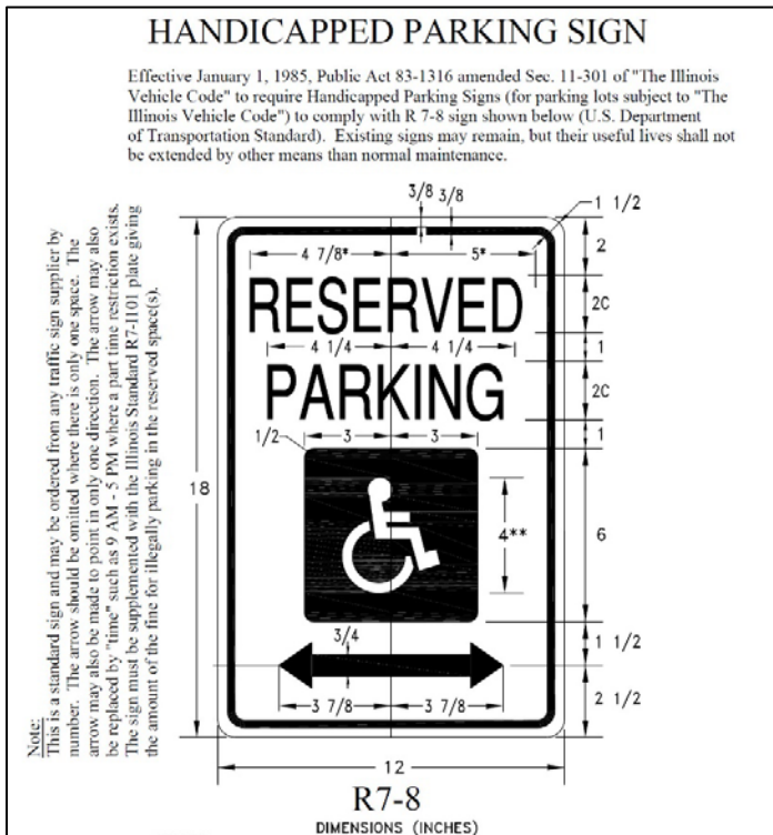
Figure 93: Accessible Parking Sign (IAC 1997)
