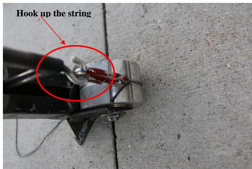
Figure C.4. Hook up the string in column B
