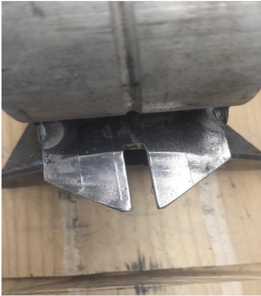
Figure 46. Improvements made for fourth generation of ISU curling and warping measurement device: shorter head of column A (top left), shorter handle of column B (top right), sharp anchor (bottom left), and replaced cord (bottom right)
