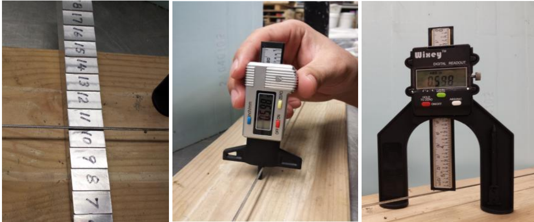
Figure 42. Comparison of the alternative rulers in the laboratory
