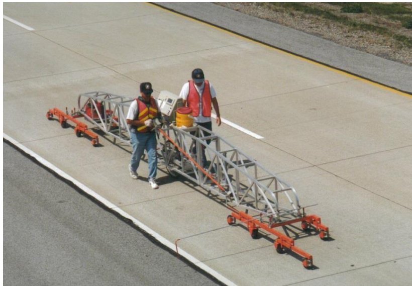
Figure 9. Typical profilograph operation
