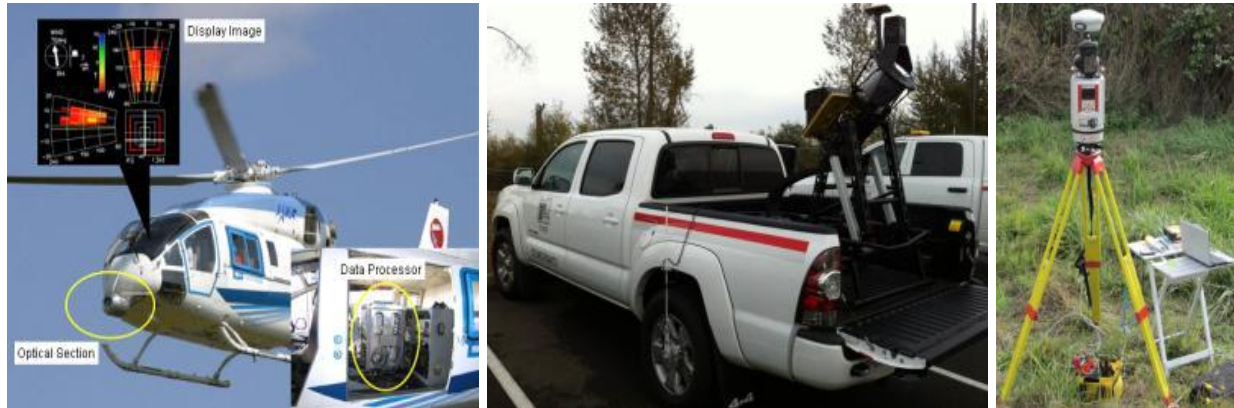
Figure 20. LiDAR systems: airborne laser scanner (left), mobile laser scanner (center), and terrestrial laser scanner (right)
