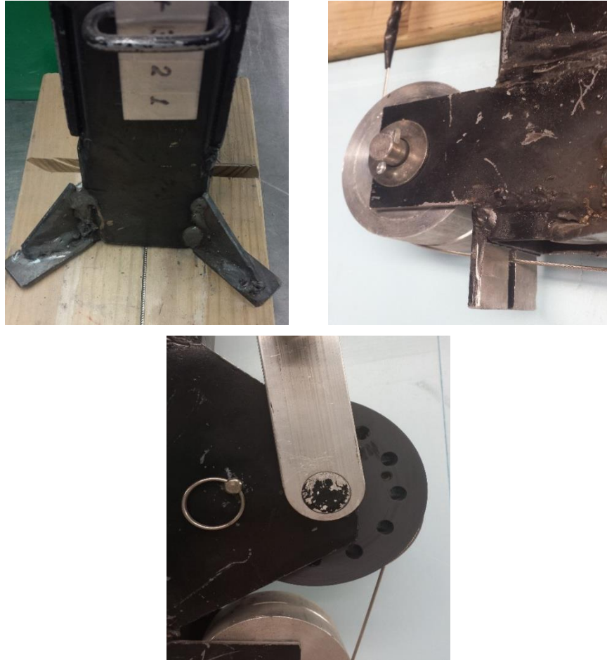
Figure 27. Improvements made for second generation of ISU curling and warping measurement device: small feet (upper left), anchor (upper right), and additional holes on the flanges of U-groove wheel in column A (bottom)
