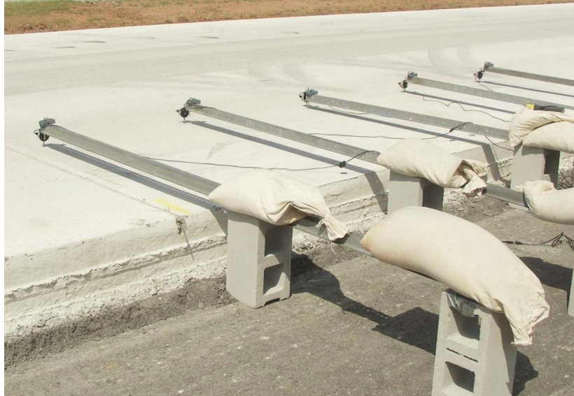
Figure 3. Digital indicators used for curling and warping measurement
