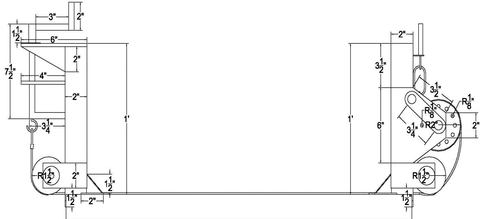
Figure B.1. Dimension diagram of ISU curling and warping measurement device
