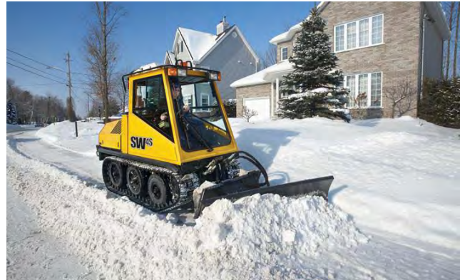
Example of a bombardier mounted with a snow plow. Vehicles like this and ATVs are used in Chicago along cycletracks that are too narrow for larger snow plow vehicles such as pickup trucks. Image credit: http://www.publiquip.com
