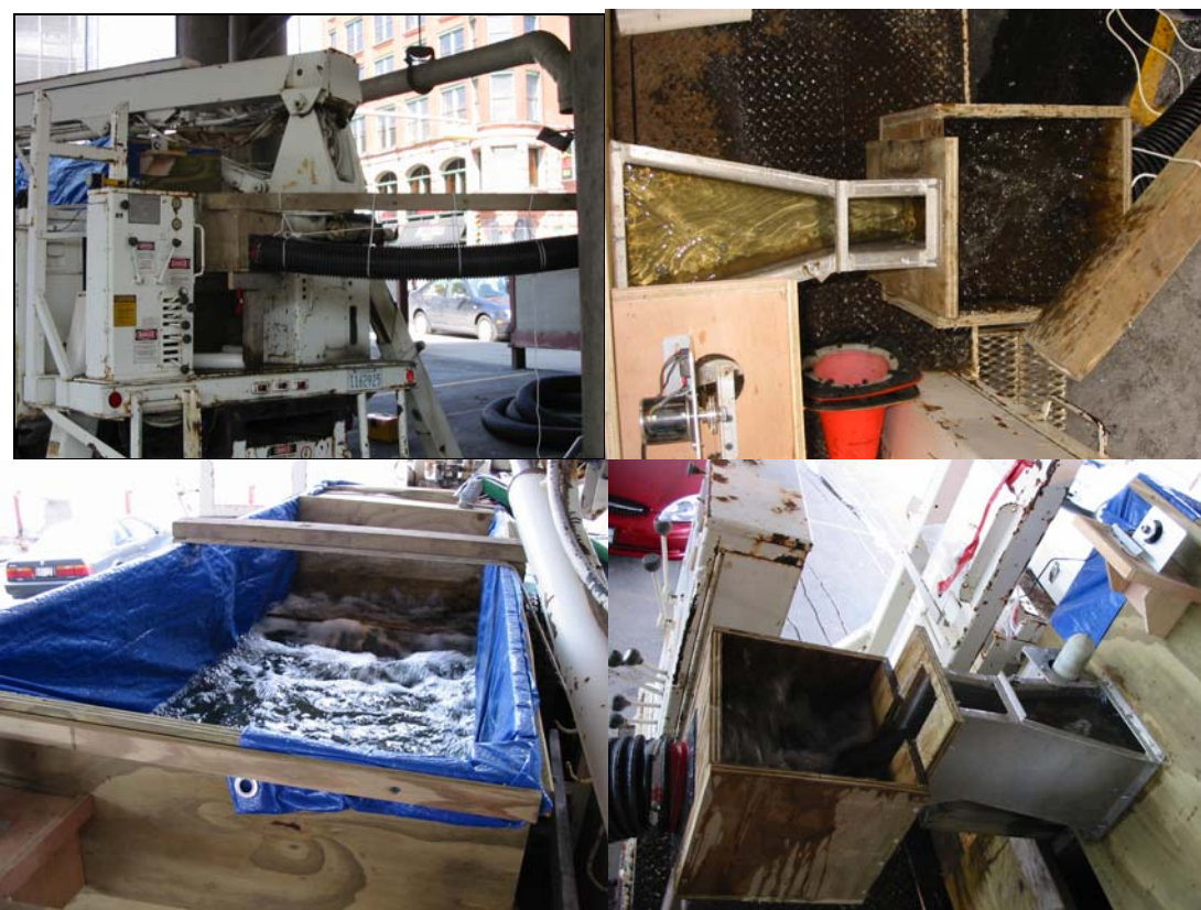
Figure 6. Flow calibration equipment: (a) boom truck, (b) approach section of the flume, (c) Parshall flume, and (d) discharge to the device.
