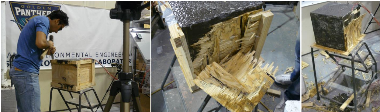
Figure A-10: Formwork removal
