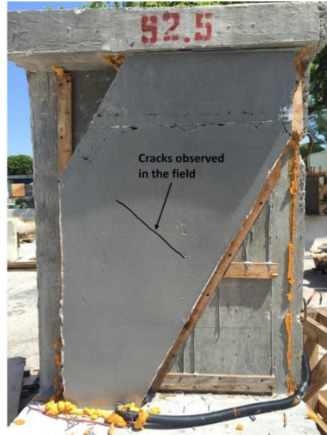
Figure 5-11: Comparison of crack locations between FEM and experimental observations for S2.5 specimen
