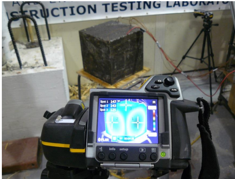
Figure A-15: Camera 2 simultaneously monitored three surface of the specimen
