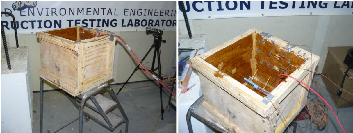
Figure A-3: Six thermocouple sensors were embedded in the neighborhood of the surface shot by the thermography Camera 1
