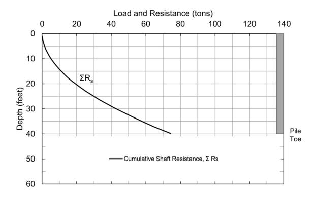
Figure 7-57 Axial load and resistance plot of cumulative shaft resistance vs. depth (after Siegel et al. 2013).
