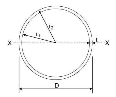
Figure 8-3 Pipe pile section dimensions.
