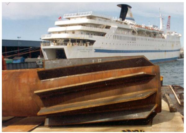
Figure 6-19 30 inch diameter Spin Fin pile.
