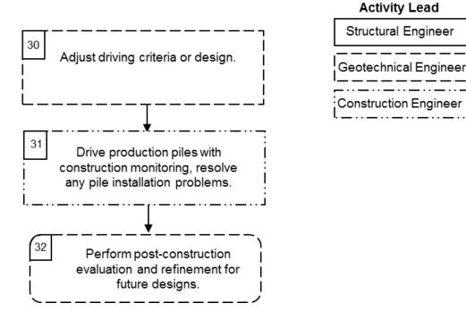
Figure 2-3 Driven pile design and construction process (continued).
