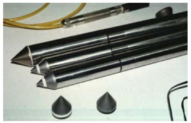
Figure 5-6 Cone penetrometers (after Mayne et al. 2001).
