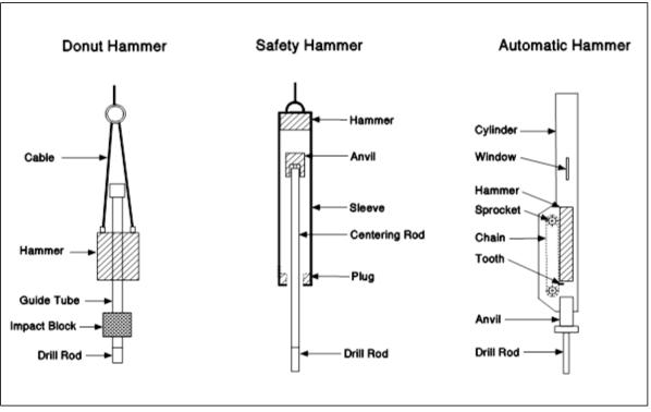
Figure 5-3 Standard Penetration Test hammer types.
