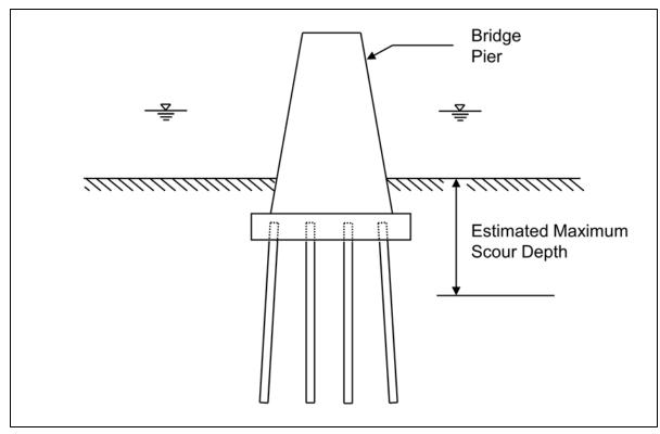
Figure 7-3 Situation where two static analyses are necessary due to scour.
