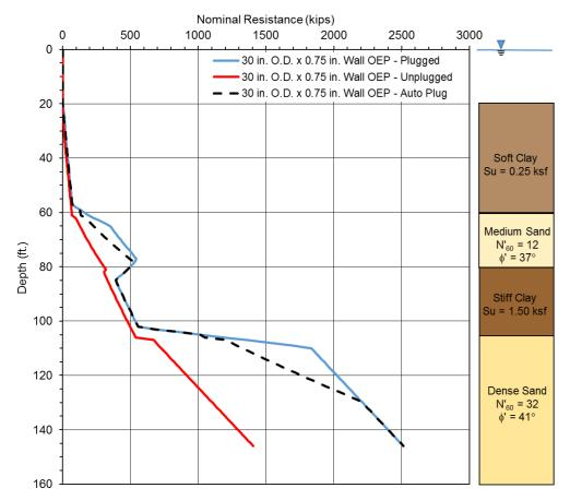
Figure 7-82 Variation in expected static resistance from APILE API method based on plugged, unplugged, and automatic calculated plugging.
