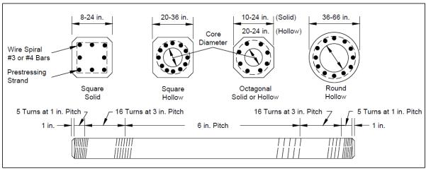
Figure 6-20 Typical prestressed concrete piles.
