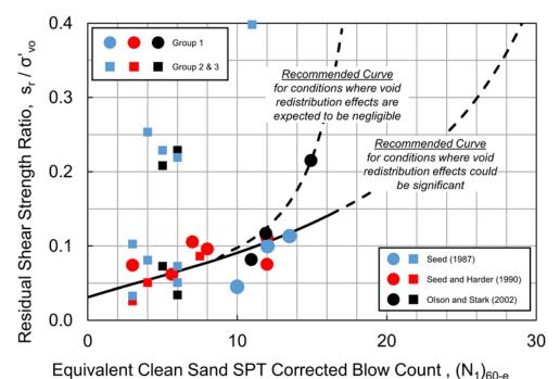
Figure 7-78 Correlation between the Residual Undrained Strength Ratio,  $s_r / \sigma'_{\infty}$  and equivalent clean sand SPT blow count,  $(N_1)_{60-e}$  (Idriss and Boulanger 2007).
