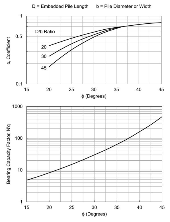
Figure 7-16 Chart for estimating  $\alpha_t$  coefficient and bearing capacity factor N'<sub>q</sub> (after Bowles 1977).
