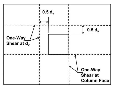
Figure 8-11 One-way beam shear critical sections from column.
