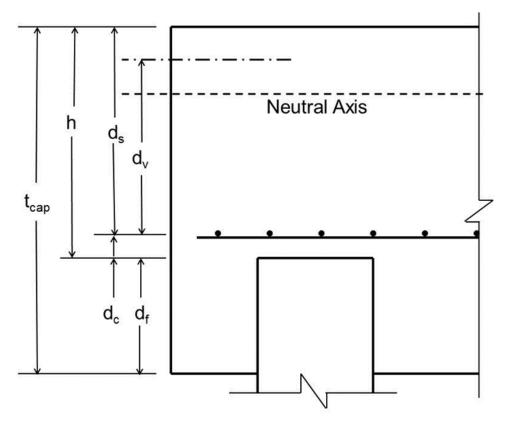
Figure 8-7 Cap section and notation.
