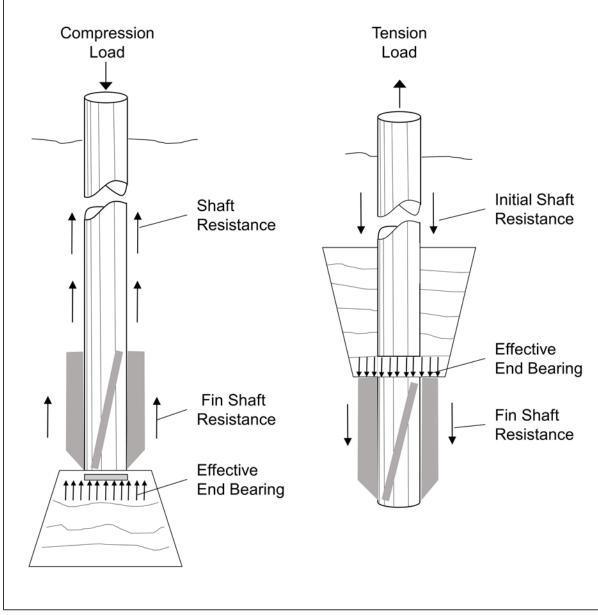
Figure 6-18 Spin Fin pile load transfer illustration.
