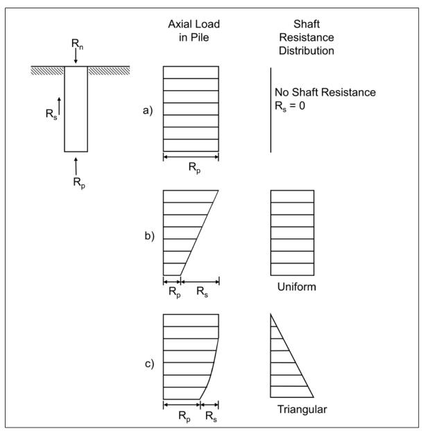
Figure 7-5 Typical load transfer profiles.
