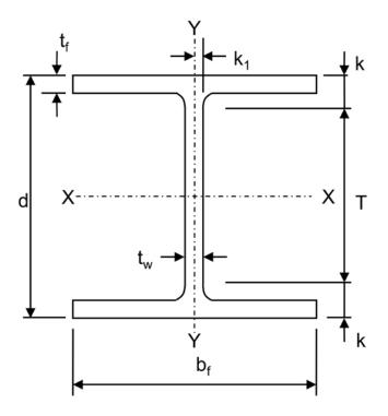
Figure 8-1 H-pile section dimensions.
