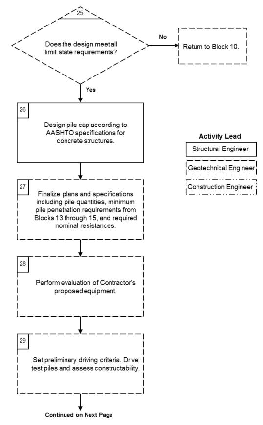
Figure 2-3 Driven pile design and construction process (continued).
