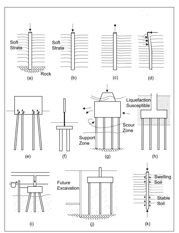
Figure 3-1 Situations in which deep foundations may be needed (modified from Vesic 1977).
