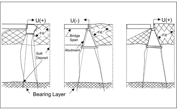
Figure 7-76 Examples of abutment tilting due to lateral squeeze.
