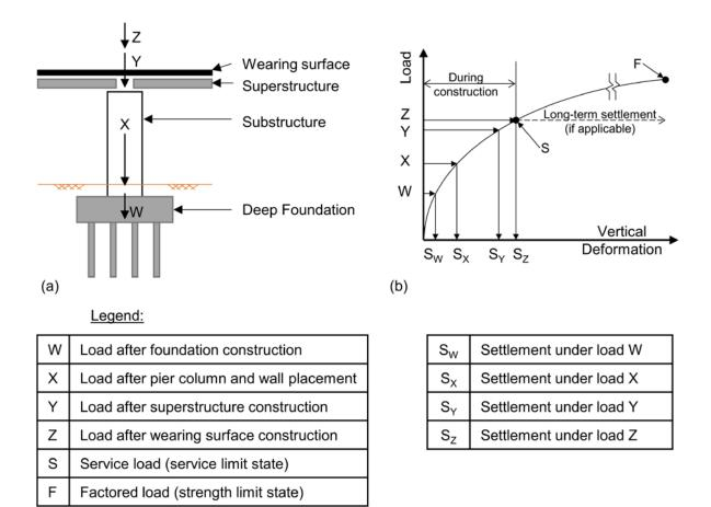
Figure 7-40 Construction point concept: (a) identification of key construction points,
