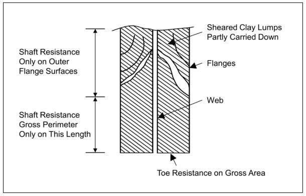
Figure 7-84 Plugging of H-piles (after Tomlinson 1994).
