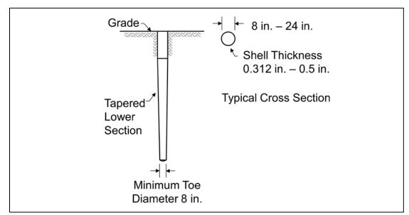
Figure 6-7 Tapertube pile typical illustration.
