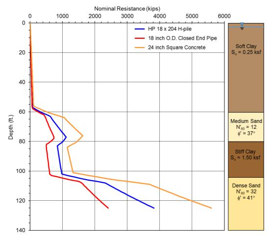
Figure 7-27 Nominal resistance versus depth for three pile types calculated by the APILE program with the FHWA Method.
