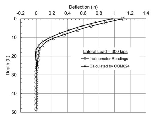
Figure 7-69 Comparison of measured and COM624P predicted load-deflection behavior versus depth (after Kyfor et al. 1992).
