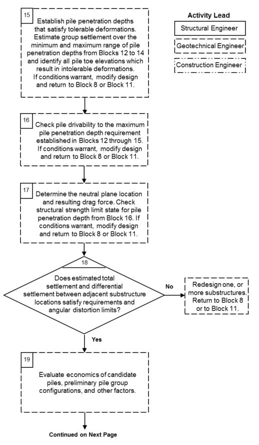
Figure 2-3 Driven pile design and construction process (continued).
