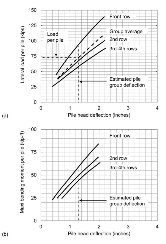
Figure 7-74 Typical plots of (a) Load versus deflection and (b) Bending moment versus deflection for pile group analysis (adapted from Brown and Bollman 1993).
