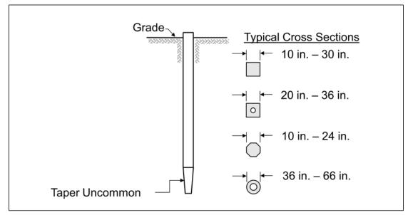
Figure 6-5 Precast, prestressed concrete typical illustration.
