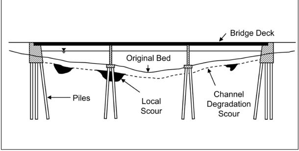
Figure 7-36 Local and channel degradation scour.
