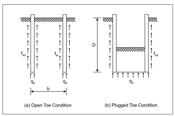
Figure 7-83 Plugging of open end pipe piles (after Paikowsky and Whitman 1990).
