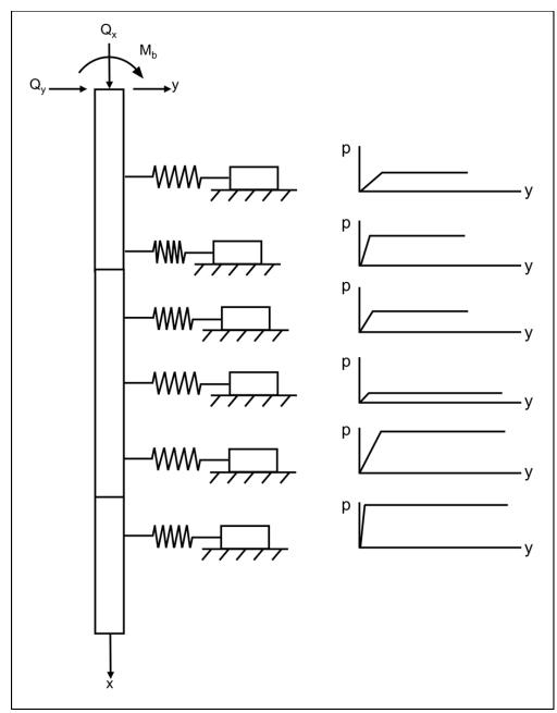
Figure 7-66 Typical lateral analysis pile-soil model.
