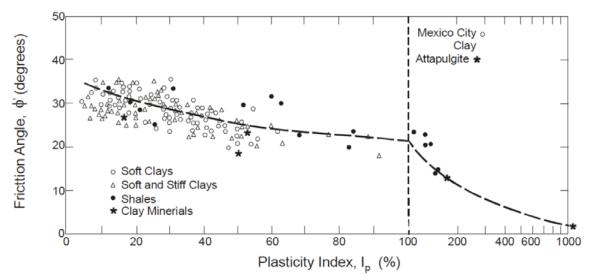
Figure 5-11 Relationship between  $\phi$ ' and PI (after Terzaghi et al. 1996).
