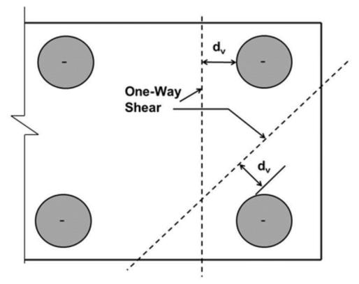
Figure 8-12 One-way beam shear critical sections from pile(s).
