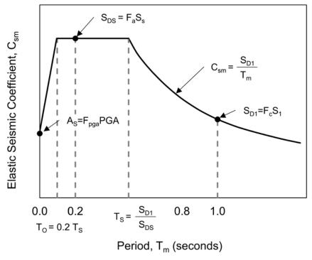
Figure 7-77 Design response spectrum (after AASHTO 2014).
