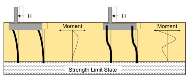
Figure 7-65 Effect of pile head fixity on moment in piles at strength limit state (after Wilson et al. 2006).
