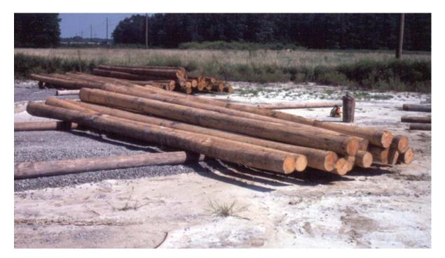
Figure 6-9 Timber piles.
