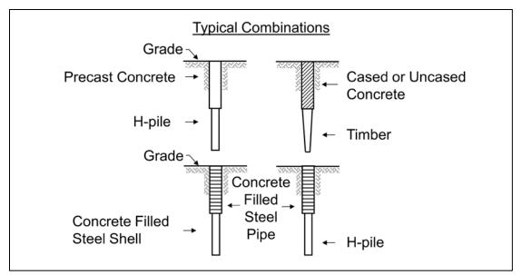
Figure 6-8 Composite piles typical illustration.
