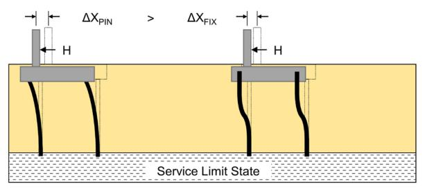
Figure 7-64 Effect of pile head fixity on translation at service limit state (after Wilson et al. 2006).
