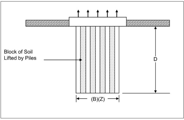
Figure 7-34 Uplift of pile group in cohesive soils (after Tomlinson 1994).
