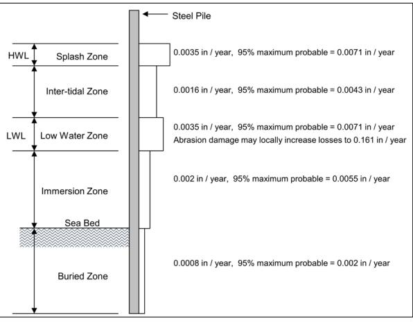
Figure 6-29 Loss of thickness by corrosion for steel piles in seawater (after Morley and Bruce 1983).
