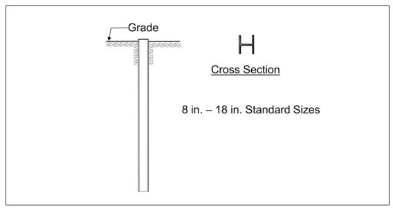
Figure 6-3 Steel H-pile typical illustration.
