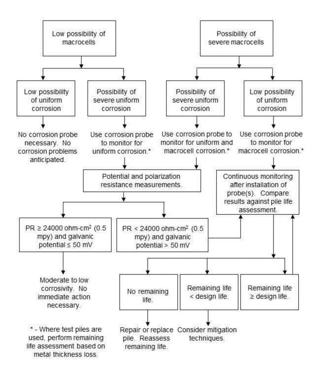
Figure 6-28 Procedure for determination of electrochemical testing, corrosion monitoring and corrosion mitigation techniques.
