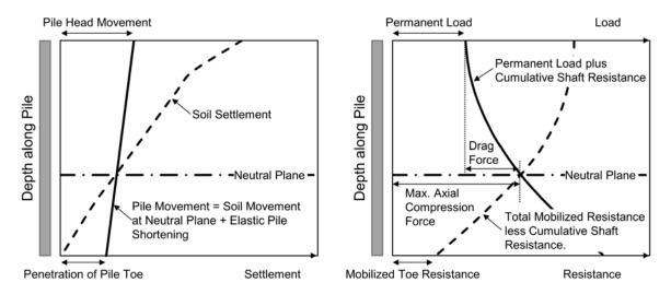
Figure 7-52 Conceptual illustration of soil and pile movement (left) and resulting neutral plane and pile forces (right) (adapted from Siegel et al. 2013).
