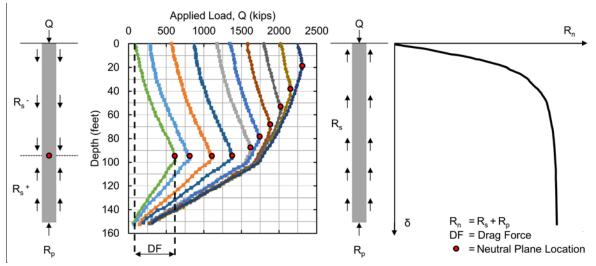
Figure 7-51 Change in neutral plane, negative shaft resistance, and drag force during transition to geotechnical strength limit (after MnDOT Geotechnical Manual).
