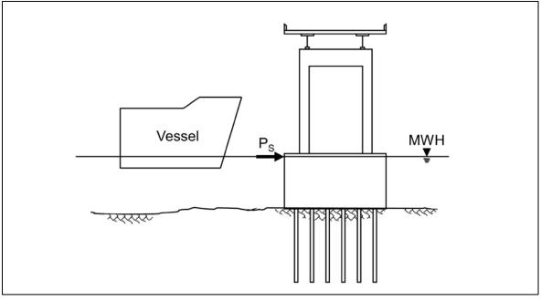
Figure 7-79 Application of equivalent impact force (after AASHTO 2014).
