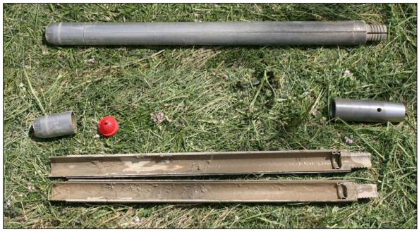
Figure 4-2 Standard split spoon sampler.
