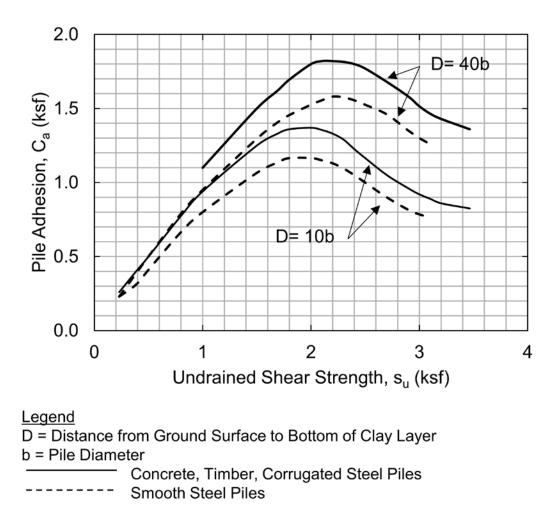
Figure 7-17 Adhesion values for piles in cohesive soils (after Tomlinson 1979).
