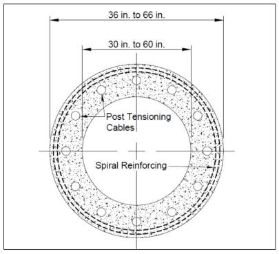
Figure 6-22 Typical spun-cast concrete cylinder pile section.
