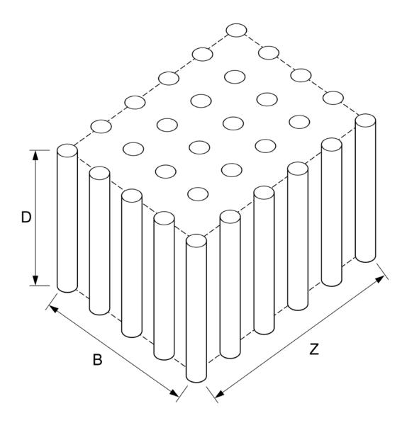
Figure 7-31 Three dimensional pile group configuration (after Tomlinson 1994).
