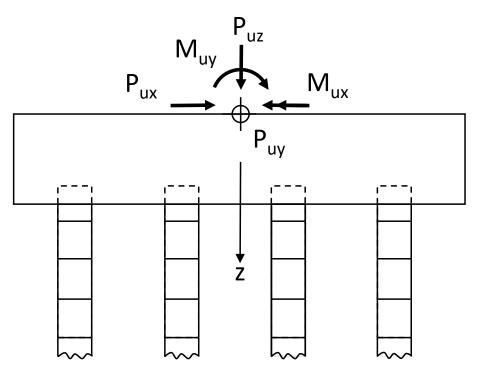
Figure 8-6 Pile group layout. (Note: Column supported on pile cap not shown for clarity)
