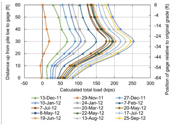
Figure 7-50 Calculated load versus depth in 12.75 inch O.D. concrete filled pipe pile as a function of time (after MnDOT Geotechnical Manual).
