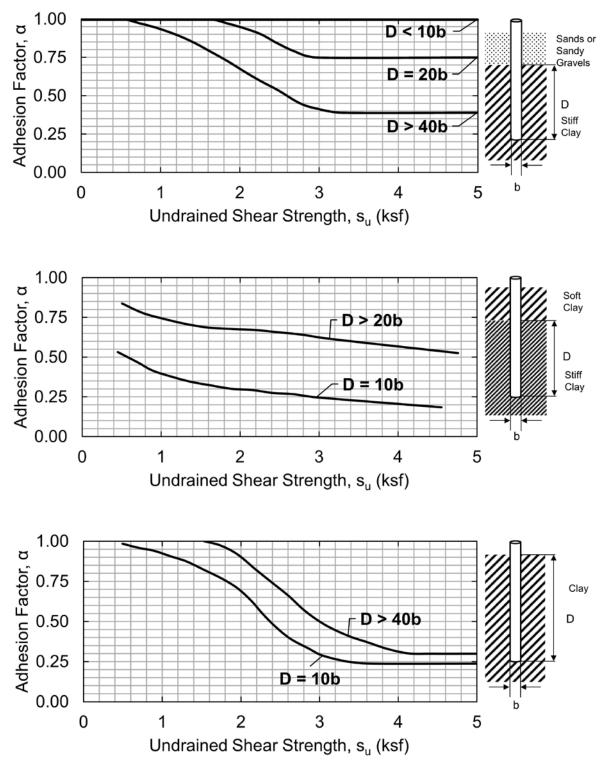
Figure 7-18 Adhesion factors for driven piles in clay (Tomlinson 1980).
