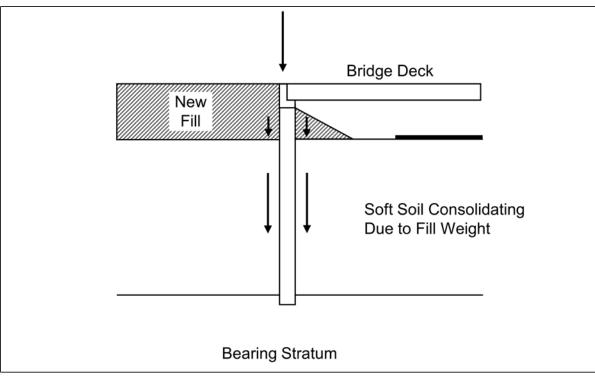
Figure 7-53 Common downdrag situation due to fill weight.
