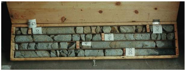
Figure 4-4 Rock core samples.
