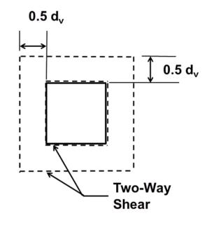
Figure 8-8 Critical punching (two-way) shear sections around column.
