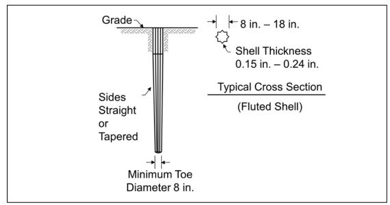
Figure 6-6 Monotube pile typical illustration.
