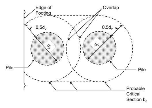
Figure 8-9 Critical section from overlapping critical perimeters (after AASHTO 2014).
