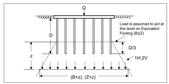
Figure 7-44 Equivalent footing concept.
