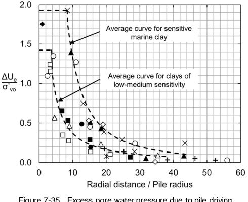
Figure 7-35 Excess pore water pressure due to pile driving (after Poulos and Davis 1980).
