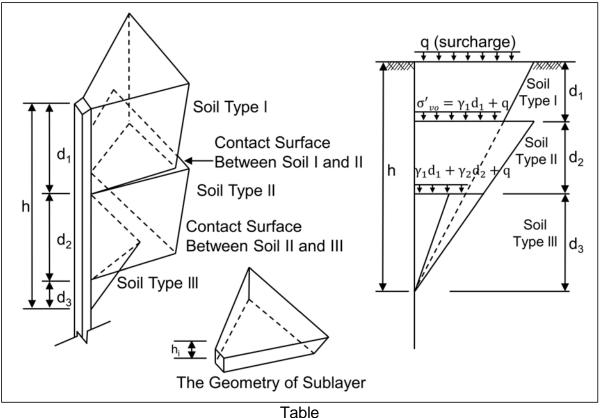
Figure 7-71 Proposed geometry of compound passive wedge (after Ashour et al. 1998a).
