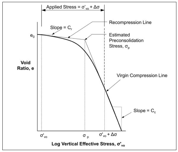
Figure 7-47 Plot of void ratio vs. vertical effective stress from consolidation test. For normally consolidated ( $\sigma'_{vo} = \sigma_p$ ) cohesive soil layers:
