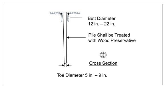
Figure 6-2 Timber pile typical illustration.
