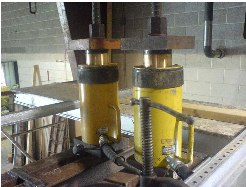
Figure 91. Photo. Hollow-core hydraulic ram bolted to the top channel beams.
