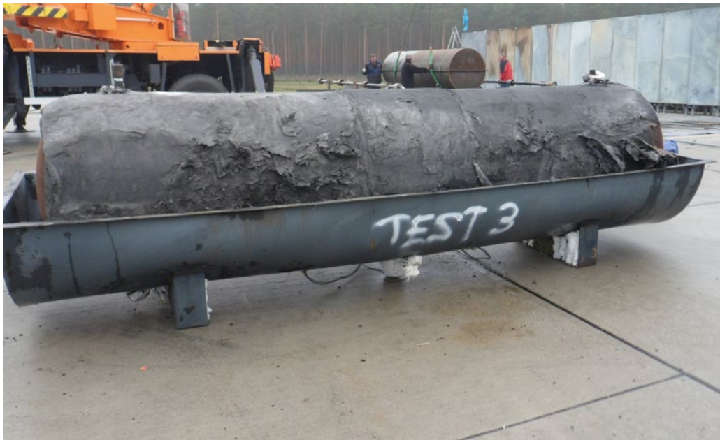
Figure 71. Test 3 with Jacket Lifted Off Note double layer of insulation at mid span
