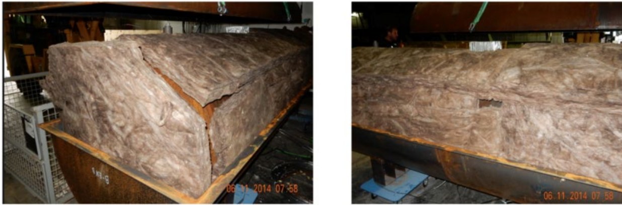
Figure 5. Insulation Before Fire Test (Test 5 Tank)
