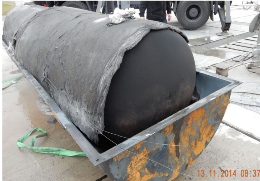
Figure 88. Test 5 with Jacket Removed. End Insulation Dropped Down
