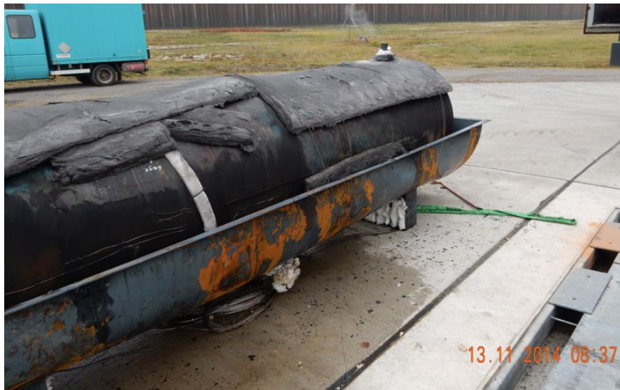
Figure 89. Test 5 with View of Side Insulation Dropped Down
