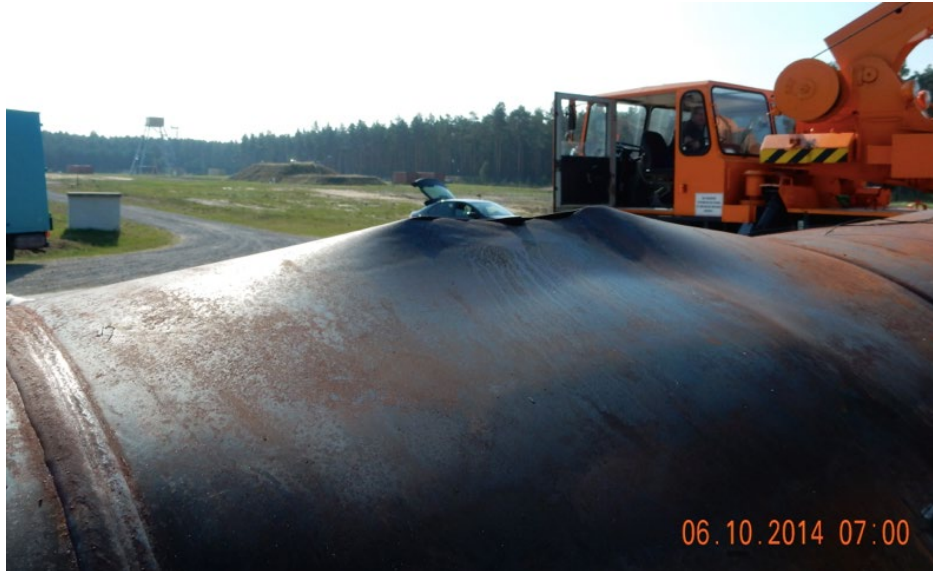
Figure 16. Test 1b - View of Vessel Rupture
