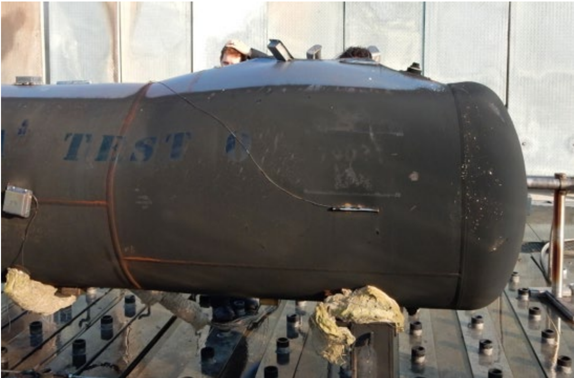
Figure 33. Test 0 - View of Deformed and Failed B-End
