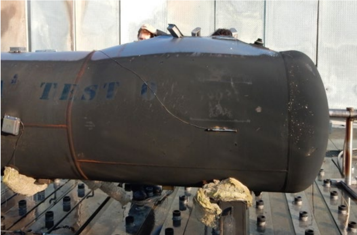
Figure 14. Test 0 - After Test - View of Deformed and Failed B-End
