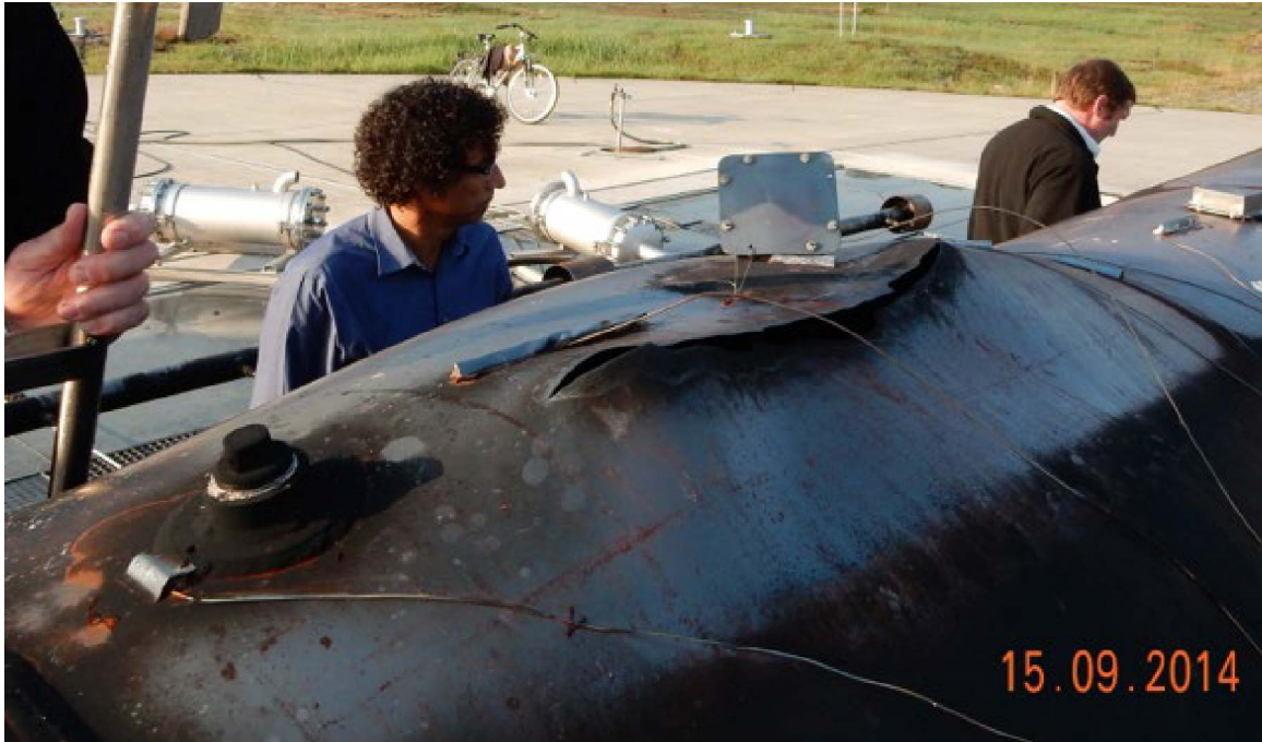
Figure 34. Test 0 - View of Deformation and Failure Opening.
