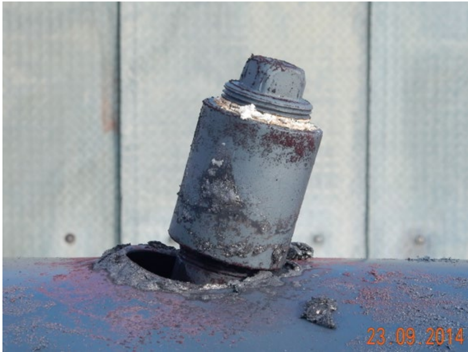
Figure 42. Test 1 - View of Damaged Fill Pipe on B-End (East) (Location of Minor Failure)
