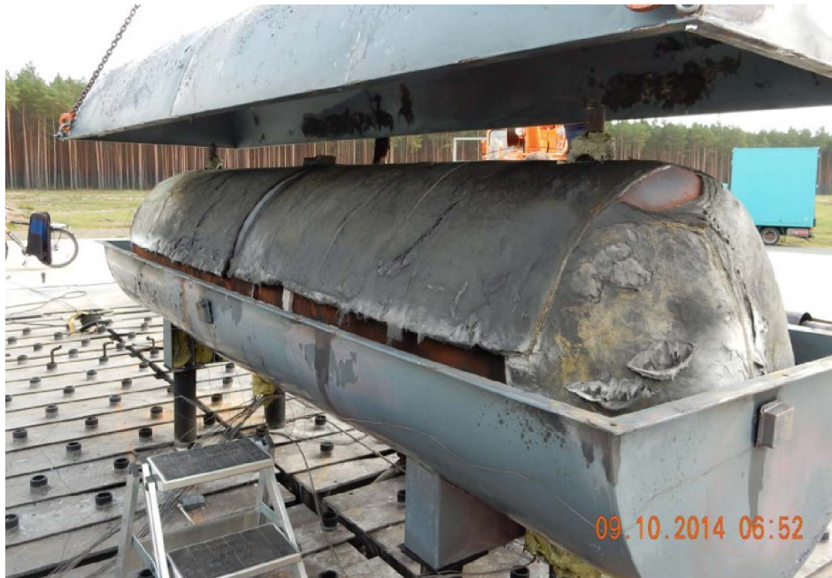
Figure 63. Test 2 - Insulation Dropped Down on Sides
