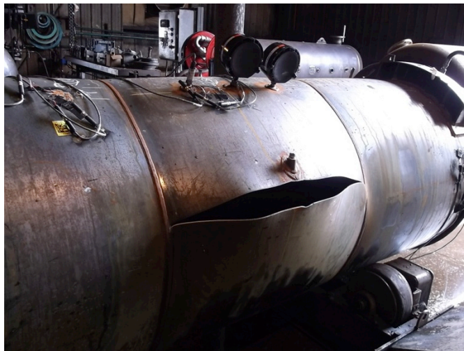
Figure 4. Burst Hydrostatic Tested Tank – Tensile Tear
