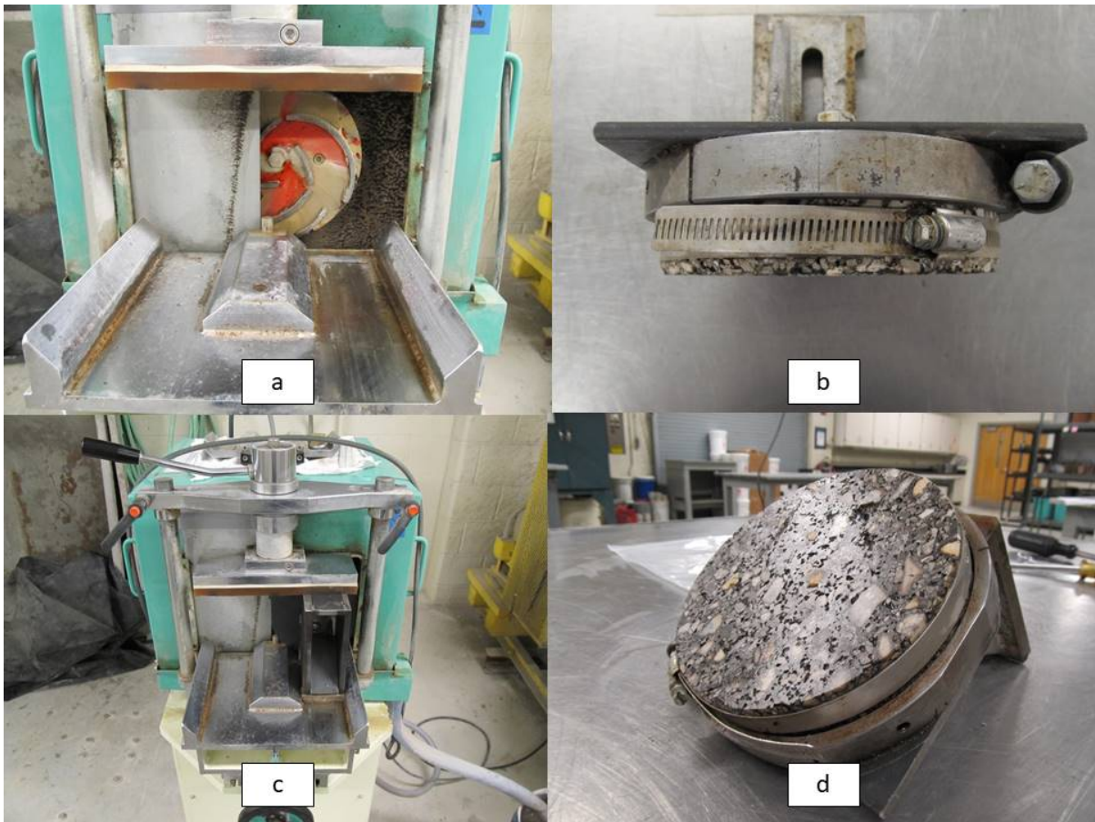
Figure 2: a) End-grinder and grinding disk b) Clamping jig with specimen in place c) Specimen being end-ground d) Specimen after grinding
