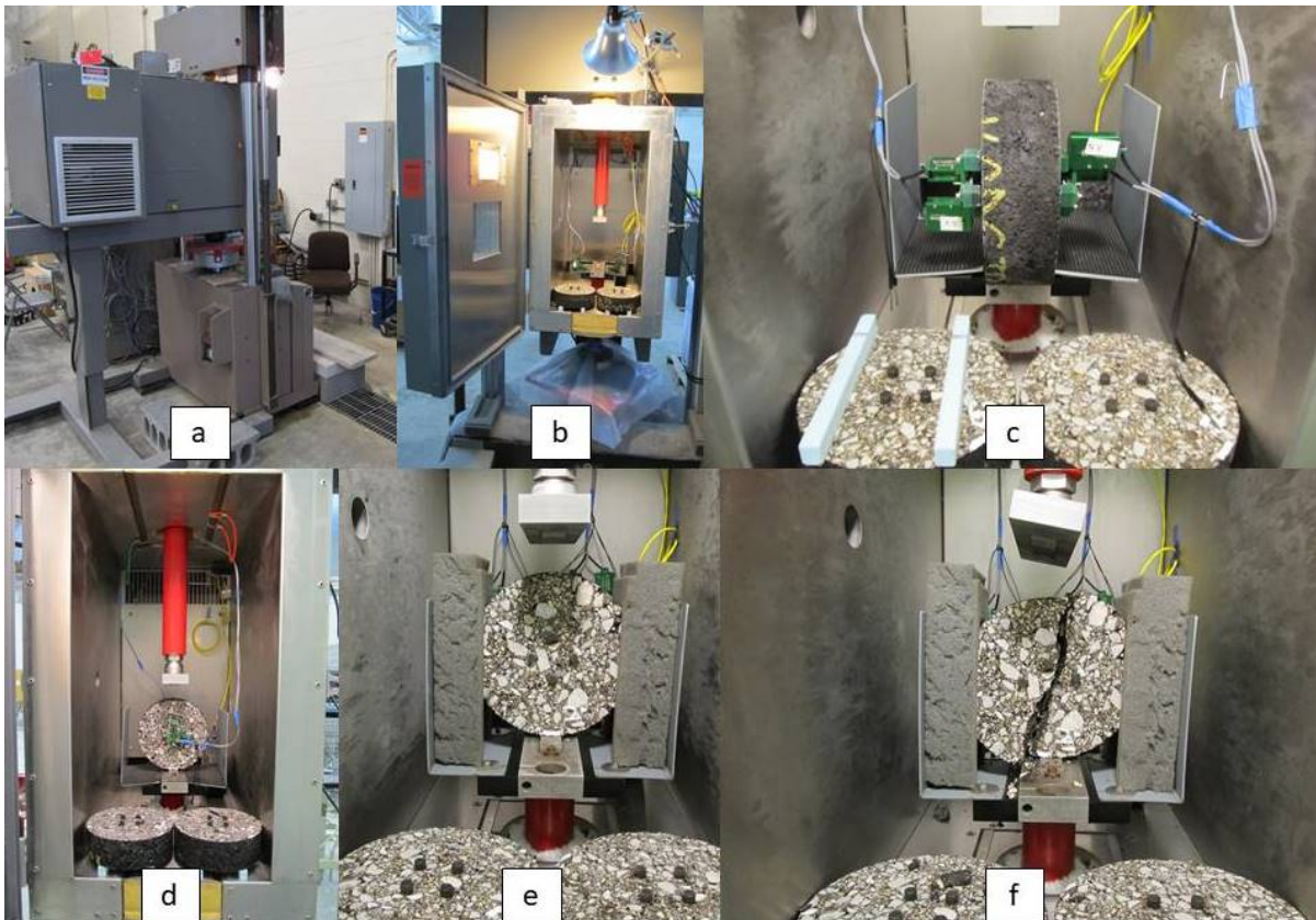
Figure 5: a) MTS 880 & temperature chamber b) Inside temperature chamber c) Extensometers on both sides of specimen d) Creep compliance setup e) IDT strength setup f) IDT strength post-failure
