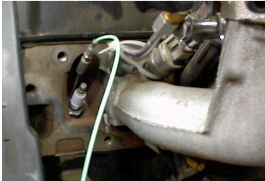
Figure 14. Modified spark plug with pressure transducer installed.
