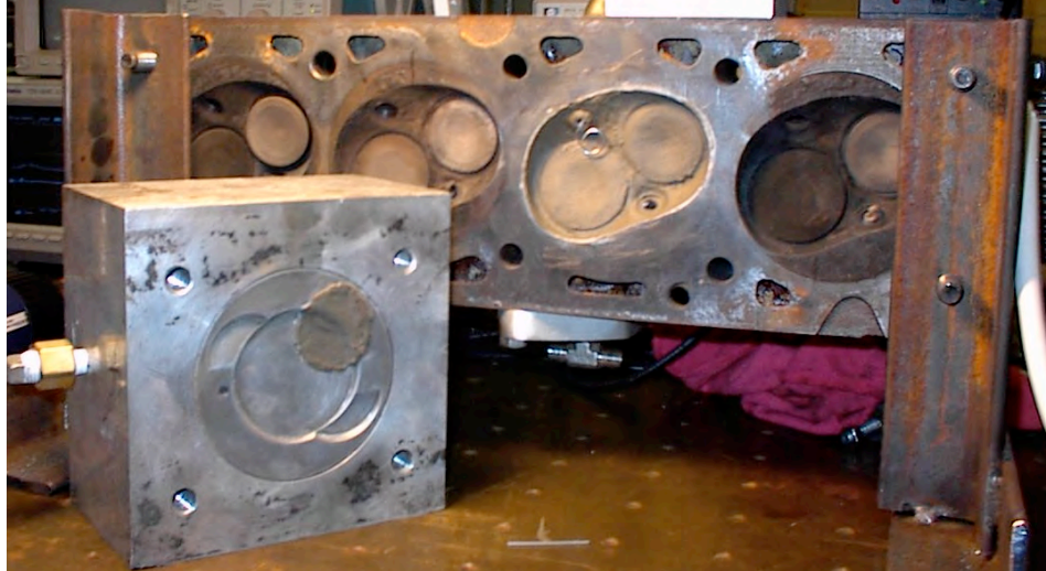
Figure 9. Test chamber using piston and cylinder head from engine (disassembled).
