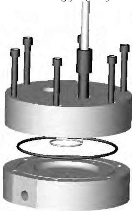
Figure 6. Exploded view of Engine Cylinder Test chamber assembly, shown with circular ring electrode
