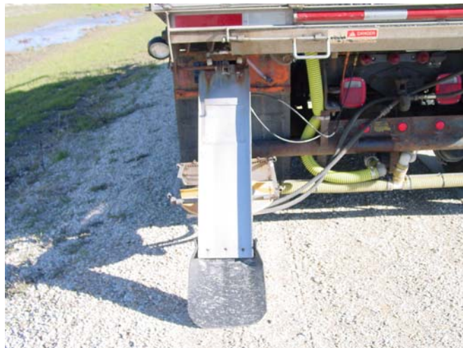
Figure 2.3. Truck B - standard truck outfitted with a shop made stainless steel chute system. The chute is designed to place material in a narrow windrow when the chute is engaged or bypass the chute and distribute material to a traditional spreader for broader distribution, depending on the needs. The system is hydraulically controlled from the cab. For purposes of this test, the chute was fully engaged for a narrow distribution.
