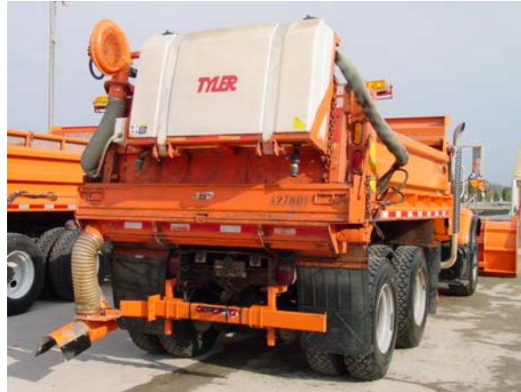
Figure 2.6. Truck E - standard truck from the Des Moines West shop equipped with one of the original Tyler zero velocity systems purchased in 1997.
