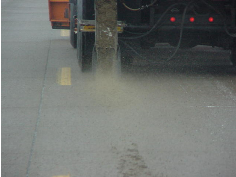
Figure 2.27. Sander chute in operation mode
