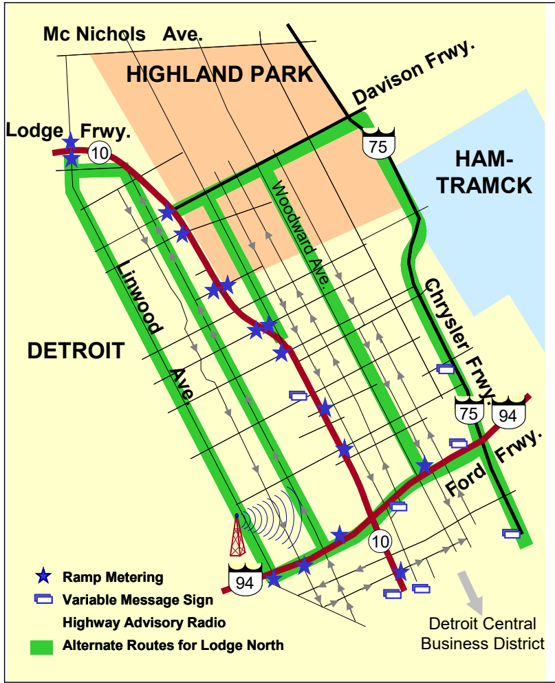
Figure B. Detroit Study Corridor Roadway and ITS Infrastructure
