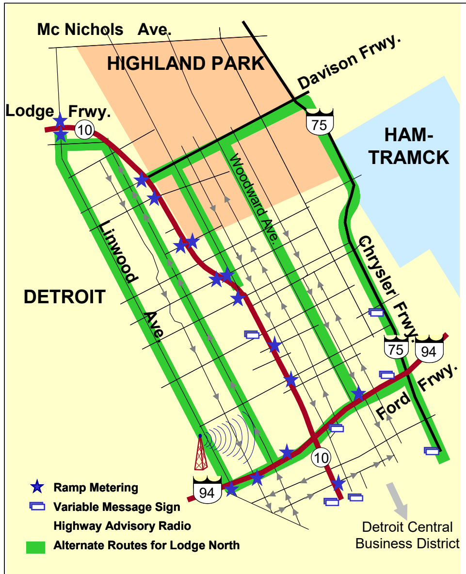
Figure 6. Detroit Study Corridor Roadway and ITS Infrastructure
