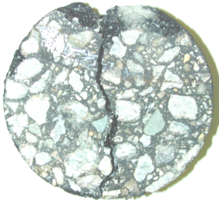
Fig. 4.11 Typical splitting failure in dynamic IDT testing
