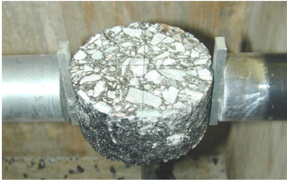
Fig. 4.8 Dynamic indirect tensile test setup in SHPB apparatus
