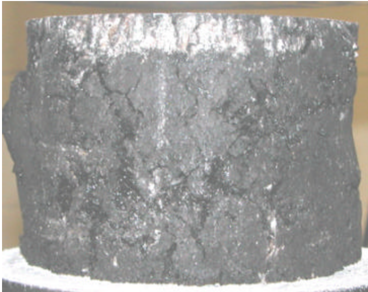
Fig. 3.9 Failed specimens from uniaxial compression testing
