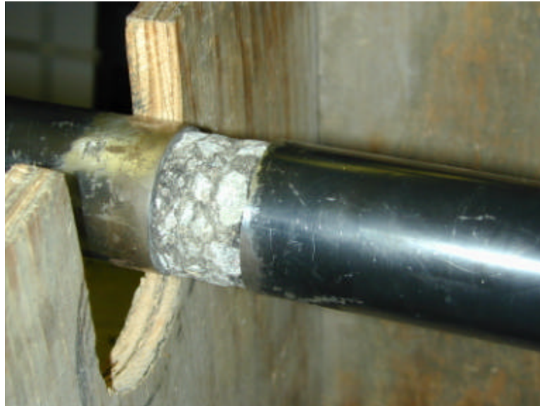
Fig. 4.3 Dynamic compressive testing setup with specimen between bars
