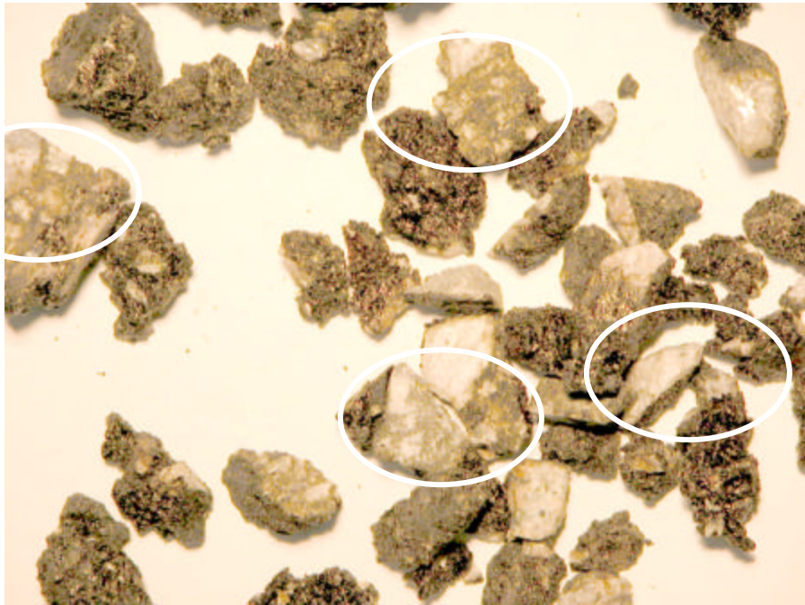
Fig. 4.13 Failure pattern from dynamic compression testing (fractured aggregates marked with circles)
