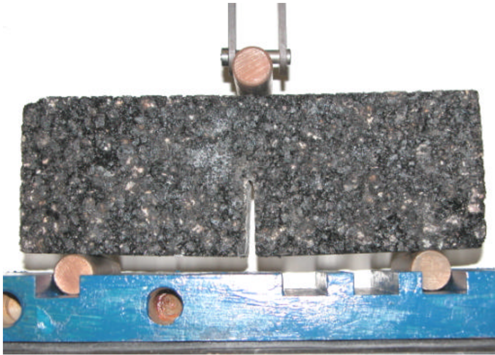
Fig. 5.5 Setup for testing quasi-static fracture behavior
