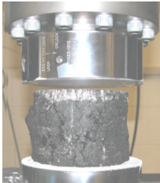
Fig. 3.2 Setup for static compression testing
