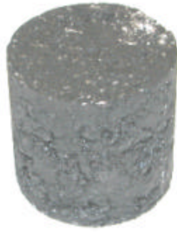
Fig. 3.1 Specimen photograph – quasi-static compression
