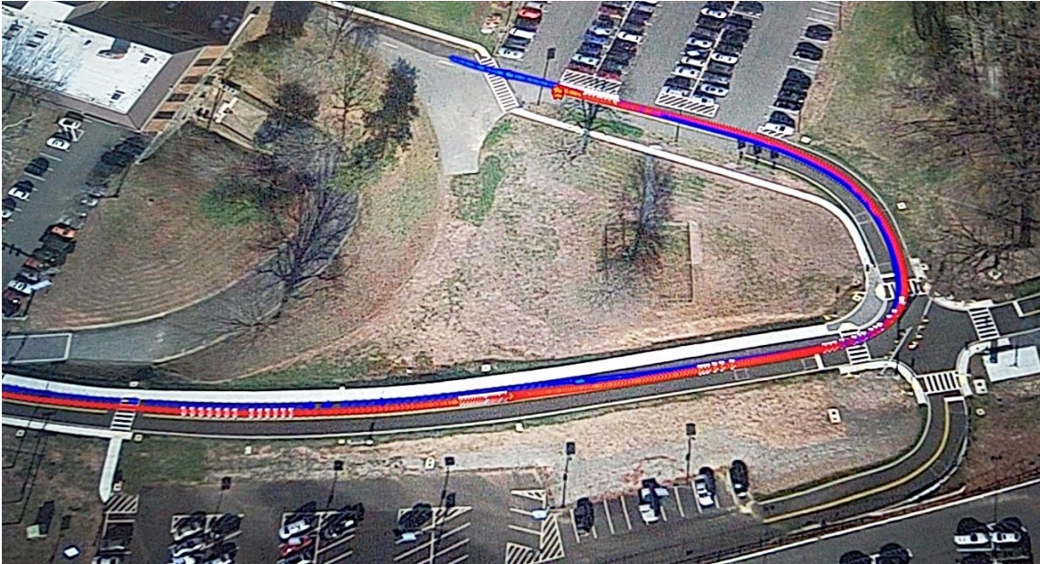
Figure 15. Visualization of GPS Accuracy from a Wyoming Test Run (Source: Wyoming CV Pilot Site, 2018)
