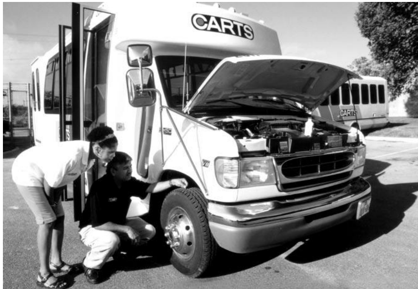
Rene Guajardo, the director of safety and service quality for Capital Area Rural Transportation System (CARTS), shows Linda Mainor how to perform a pre-trip inspection before she begins her bus route. CARTS drivers perform a daily inspection of their buses, including a check of various items in the engine compartment, the driver's area, operational lights, brakes and suspension, passenger area, wheel chair lift and then a general walkaround.
