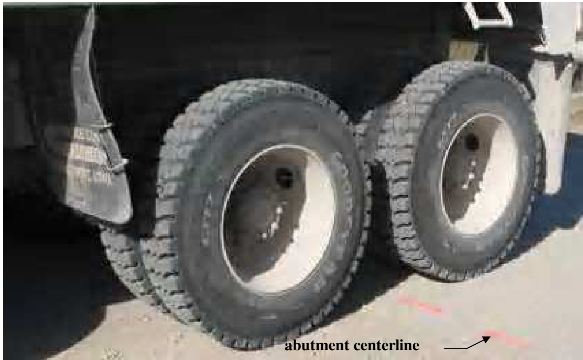
Figure 3.11. BCB Truck Tandem Centroid Centered Over Abutment.
