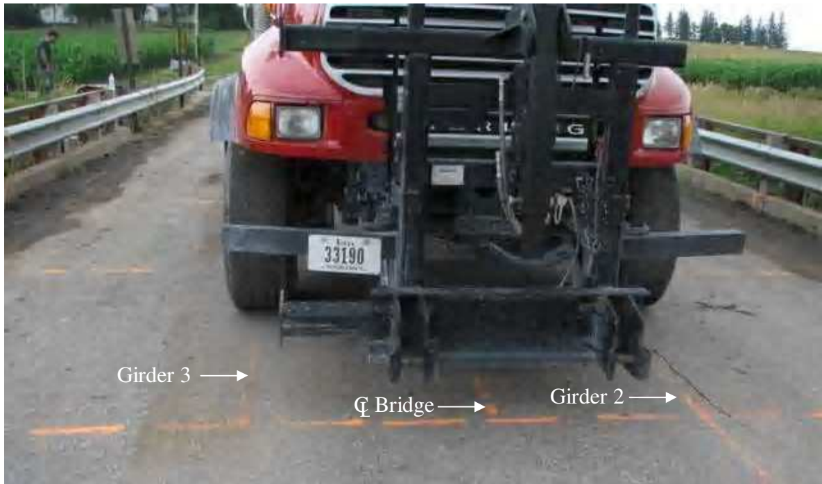
Figure 8.7. HCB Test Truck in Lane 3.
