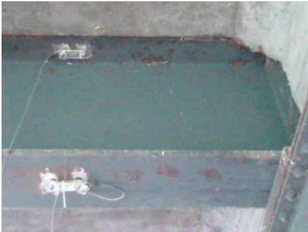
Figure 6.6. CCB Bearing Transducer Locations.
