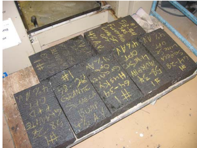
Figure 6.16. Compacted slabs before cutting
