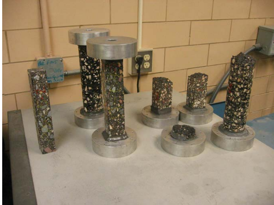
Figure 7.51. TSRST specimens with different shapes
