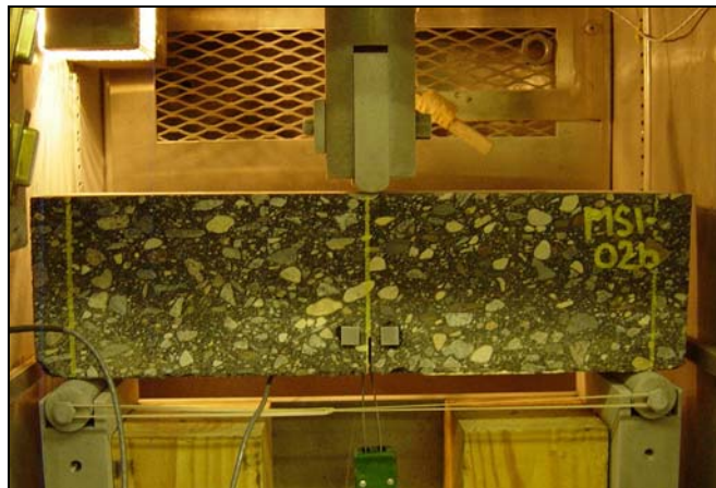
Figure 6.14. Test configuration of the SE(B)
