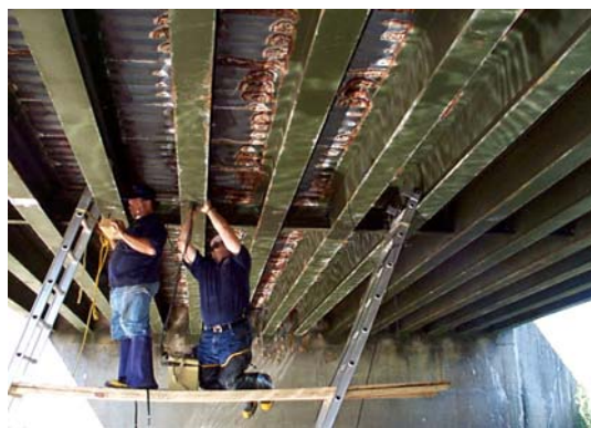
FIGURE 2: Spot Welding of Strain Gage onto Flange
