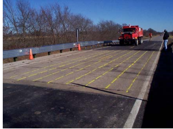
FIGURE 11: Test in Progress on FRP Deck
