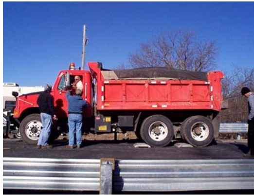
FIGURE 9: Test Load for FRP Deck Approximately 47,800 lbs
