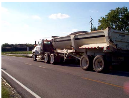
FIGURE 8: Test Load for Original Deck Approximately 78,400 lbs
