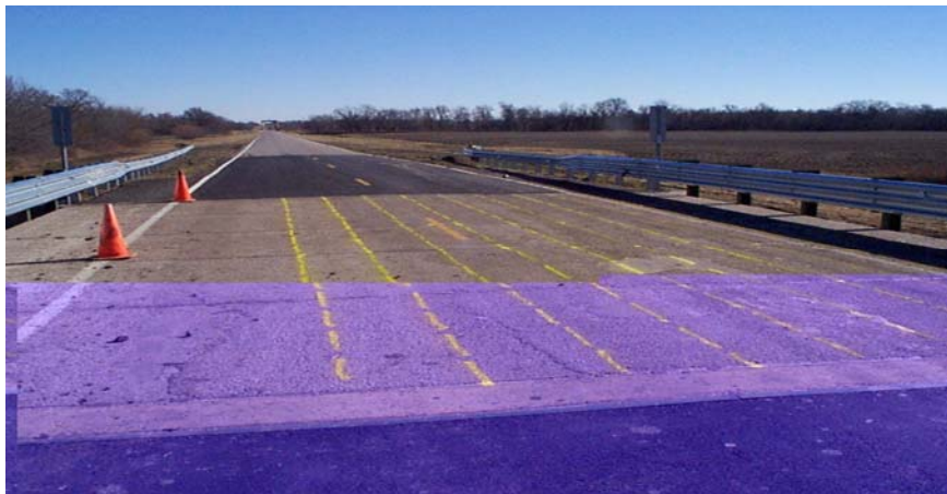
FIGURE 6: Load Pattern Layout on Bridge Deck
