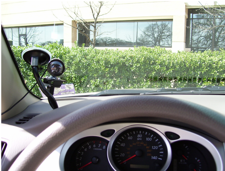
Figure 4: Windshield-mounted Driver Face Camera
