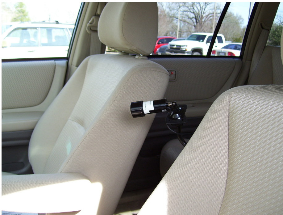
Figure 5: Center-mounted DVD View Camera
