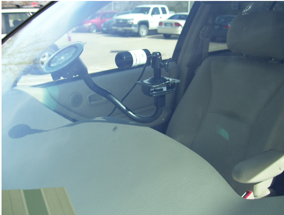
Figure 6: Windshield-mounted Forward Scene Camera
