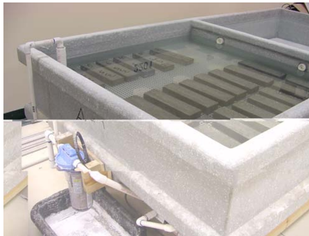
Photo 6.5.4.1-2 - To evaluate durability, ASTM C-1012 is utilized.
