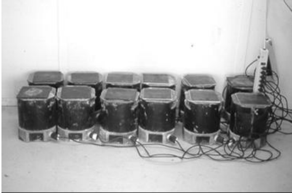
Figure 7.2.8-1 Temperature Match Curing for Prestressed Concrete Beams
