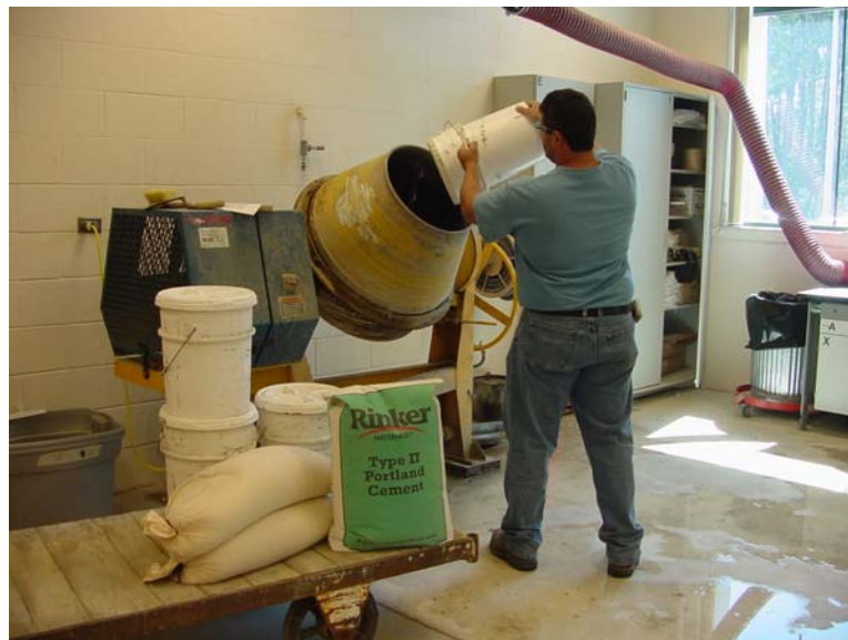
Photo 6.3.2 -2. Trial batching concrete mixtures.
