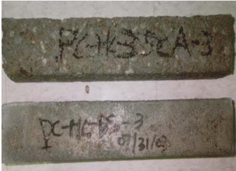
Figure 4.3 Comparison between PC-HC-35CA and PC-HC-BS Specimens after 120 cycles
