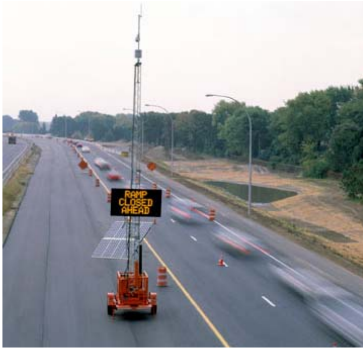
Figure 29. Portable Traffic Control Devices Can Assist with Work-Zone Activities
