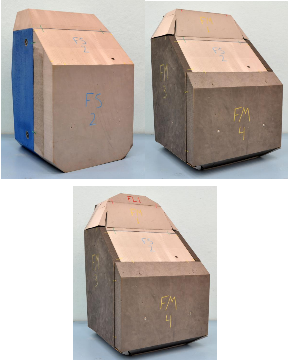
Figure 11. FF_{veh} envelope FS (left top), FM (right top), and FL (bottom).
