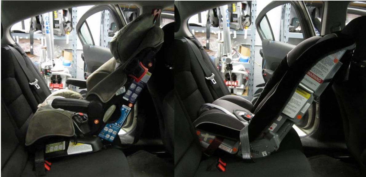
Figure 40. RF CRS that could not be installed at an acceptable angle in the vehicle.
