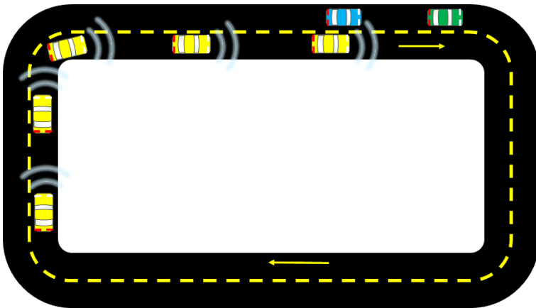
Figure 56: Interfering vehicles in yellow pass the ego vehicle in blue. The radiometer on the blue vehicle measures energy from the radars, including that which is reflected from the green target car.
