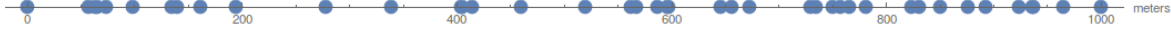
Figure 5: Locations of vehicles are shown, distributed along a line, with a Poisson point process density of 1/25 meters.
