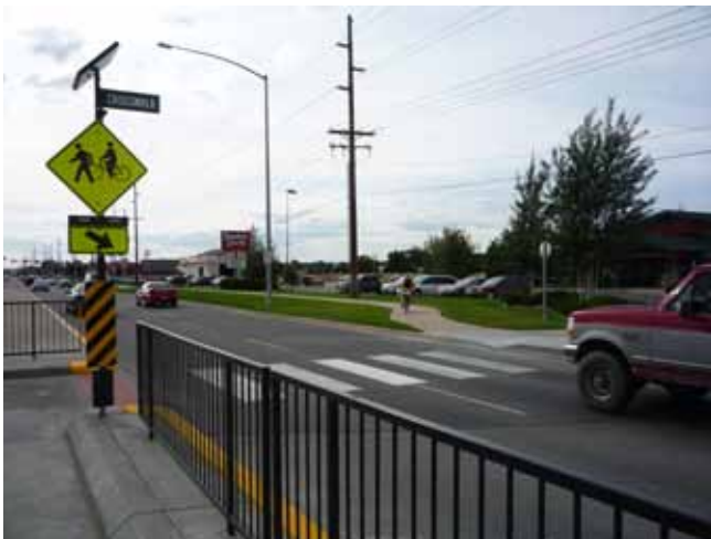
RRFB on King Avenue West in Billings
