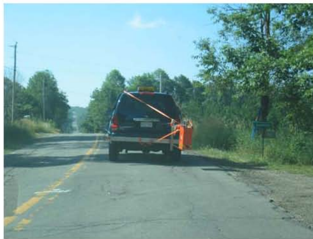
Figure 2. GPR survey with vehicle mounted antenna
