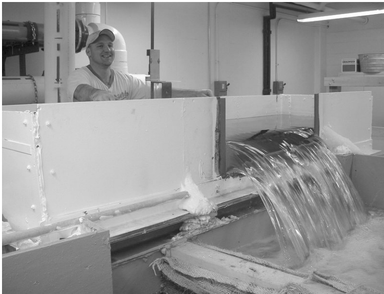
Figure 2.4: Reading the weir head
