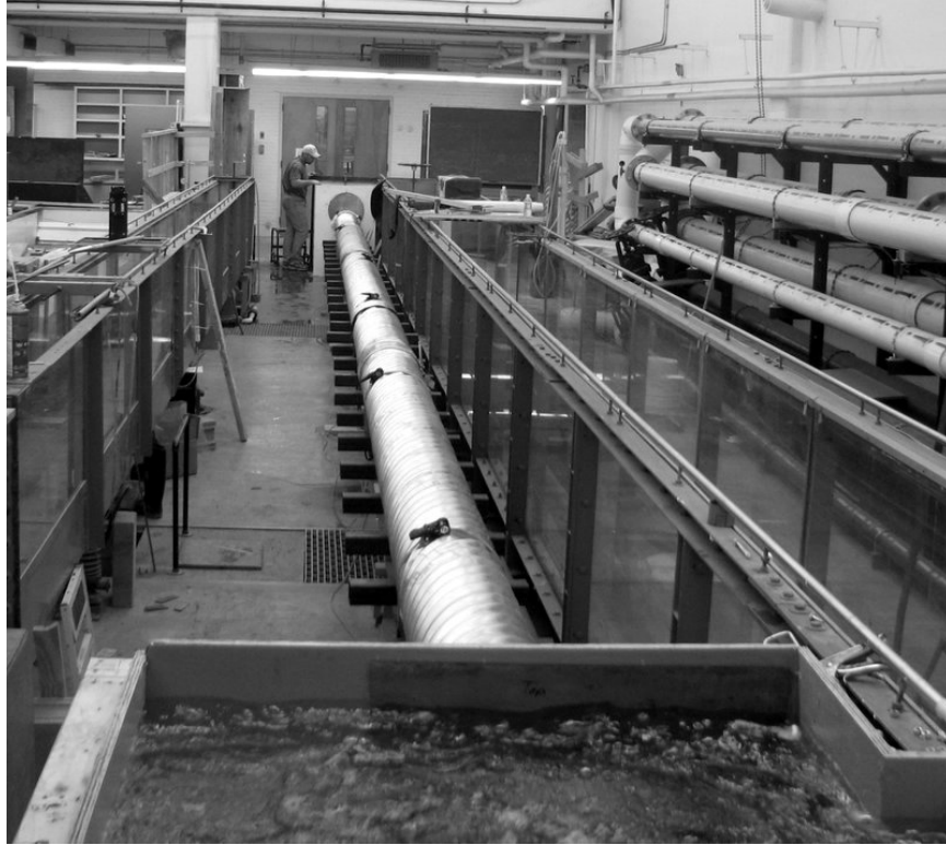
Figure 2.1: Testing the 12-inch pipe
