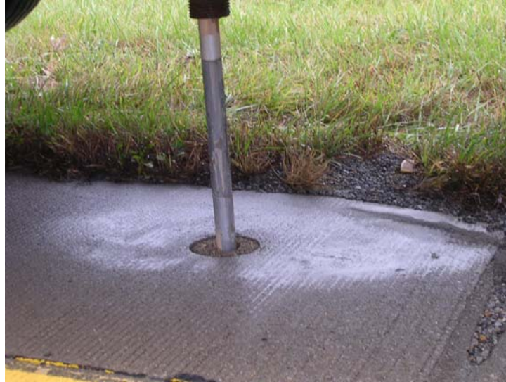
Figure 3.3: CPT Probe Pushed into Ground at Hole #2
