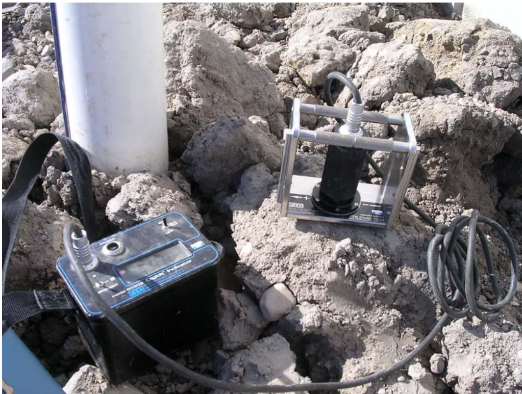
Figure 2.3: Digi-Tilt Sensor and Readout Device
