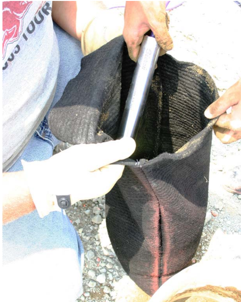
Figure 4.23 – Geotextile Bag for the Piezometer
