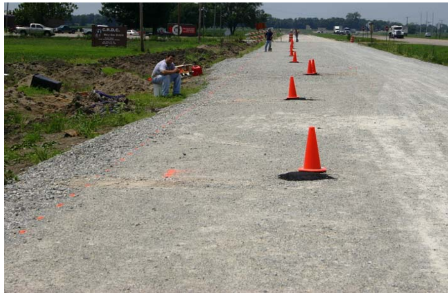
Figure 5.5 – Final Base Course with Asphalt Strain Gages
