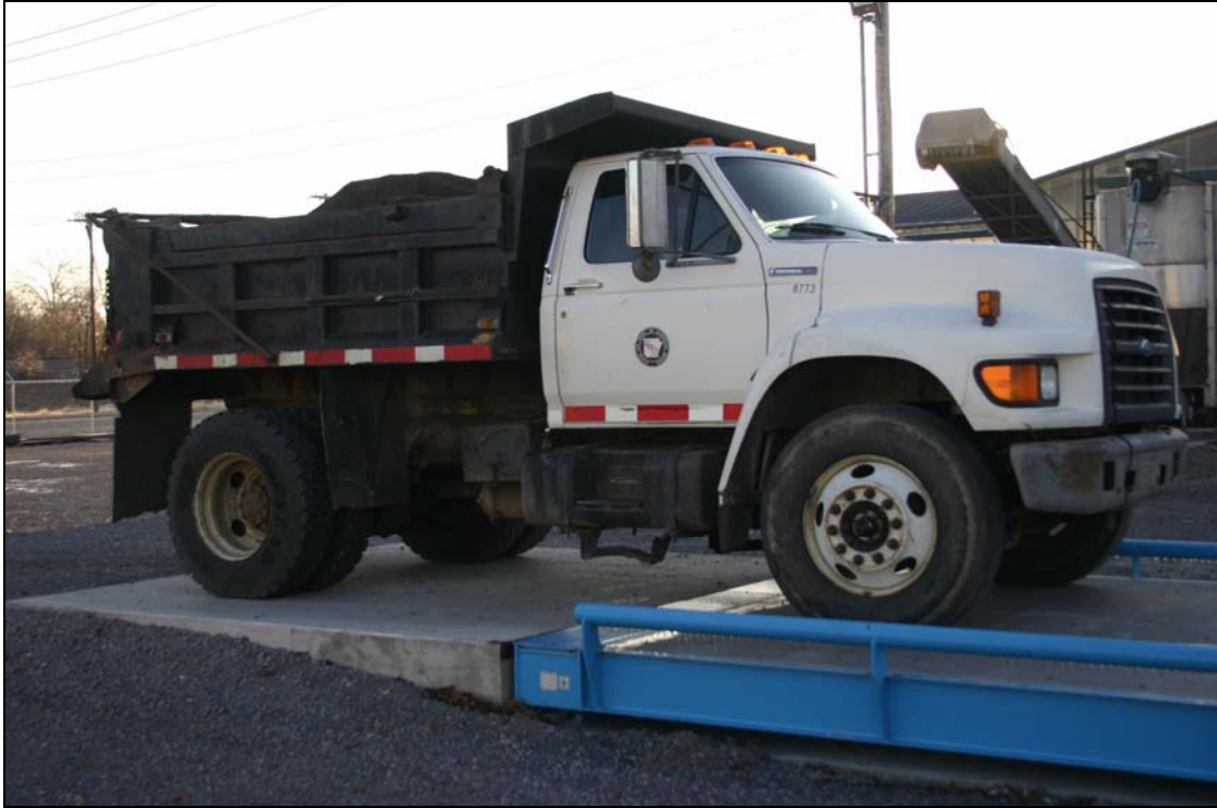
Figure 7.1 – Single Axle Dump Truck on the Scale
