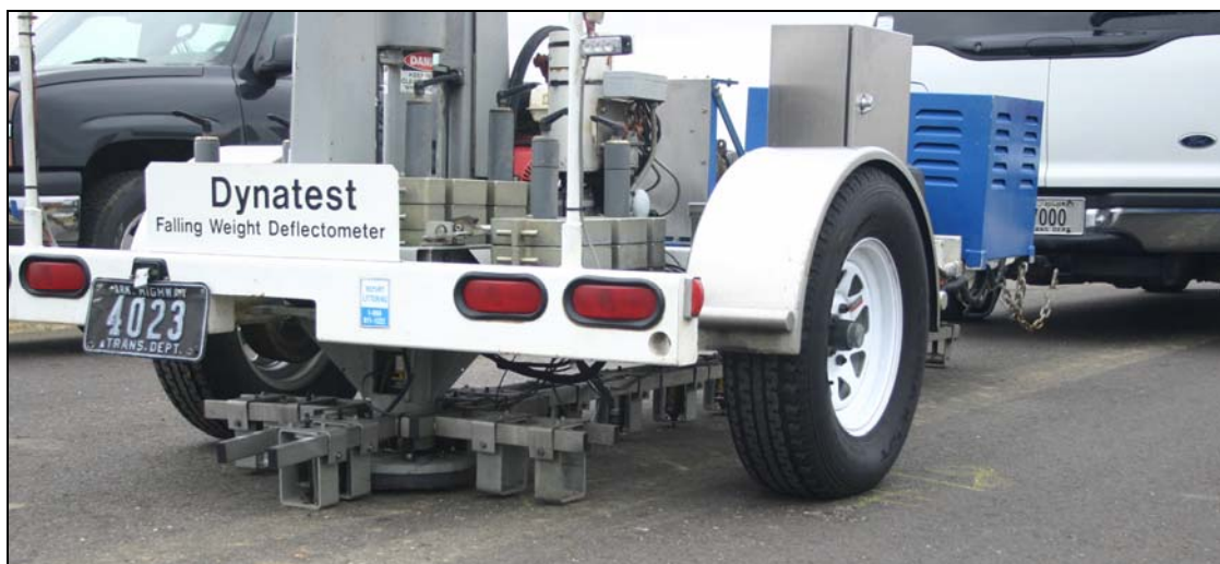
Figure 7.2 – Falling Weight Deflectometer Test
