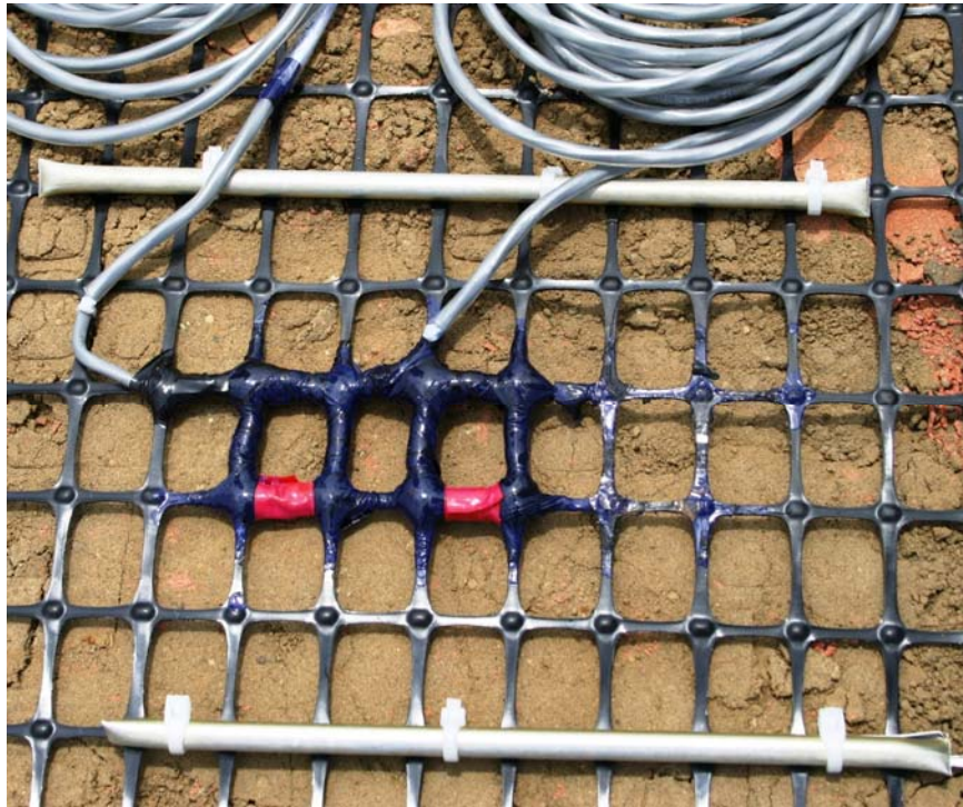
Figure 4.12 – Geogrid Strain Gage in the Field
