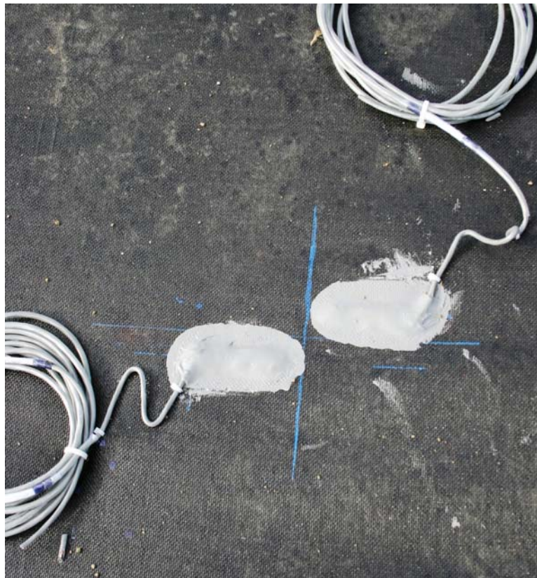
Figure 4.13 – Geotextile Strain Gage in the Field
