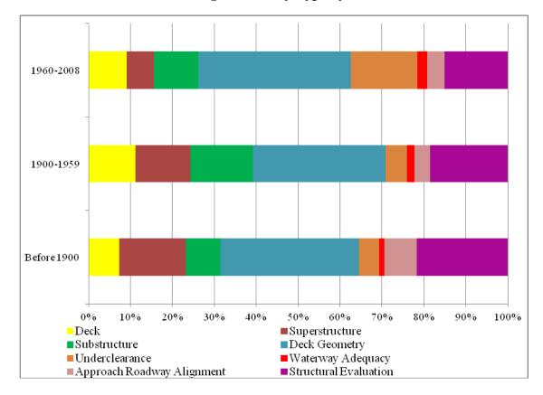
Figure 16 Distribution of Bridge by Deficiency Type and Year built
