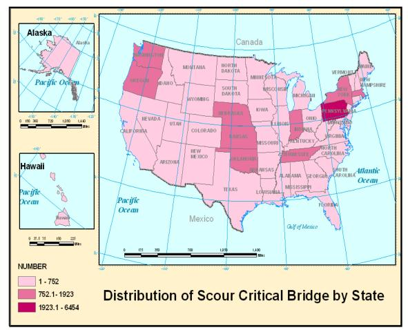
Figure 20 Distribution for Scour Critical Bridge by State (Based on template from ArcGIS)
