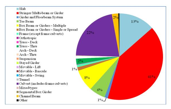
Figure 7 Distribution of Structure Types used for Main Spans of U.S. Highway Bridges, by number
