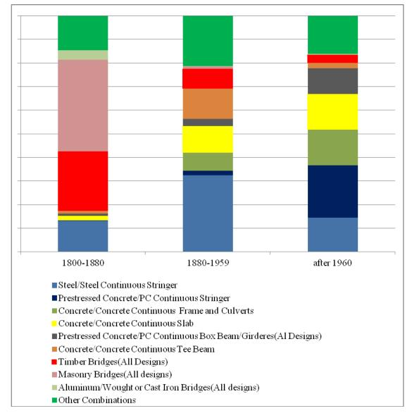
**Figure 11 Percentages of Bridges Material and Structure Type Combinations, by Time Periods**
