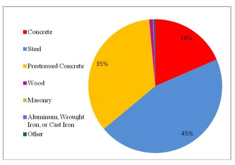
Figure 5 Distribution of Materials Used for Main Spans of US Highway Bridges, by Deck Area
