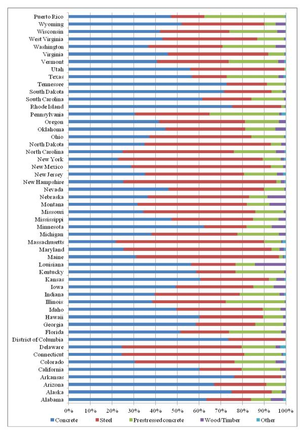
Figure 6 Distribution of Highway Bridge by Material at State Level
