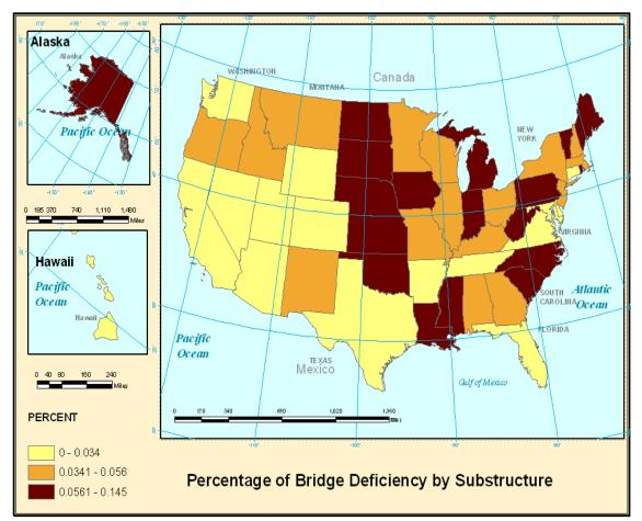
Figure 26 Distribution for Percentage of Bridge Deficiency by Substructure (Based on template from ArcGIS)
