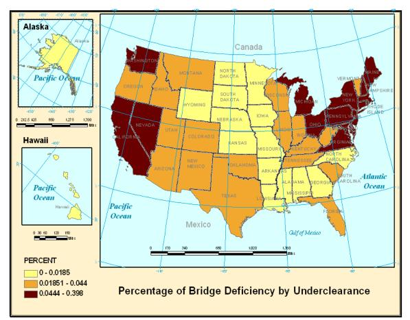
Figure 29 Distribution for Percentage of Bridge Deficiency by Underclearance (Based on template from ArcGIS)
