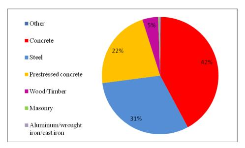
Figure 4 Distribution of Materials Used for Main Spans of US Highway Bridges by Number
