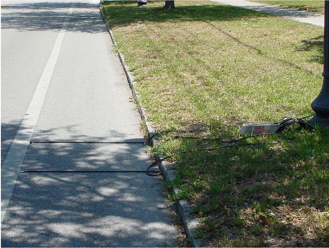
Figure 6. Typical installation of counter and tubes after bike lane installation.
