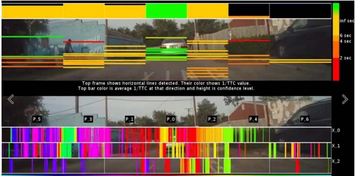
Figure 10 A live display of dangerous degree in TTC on video frames that covers all direction in front of vehicle.
