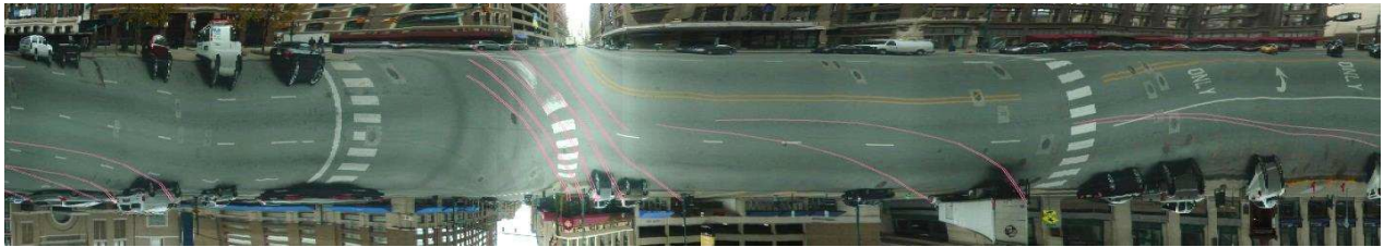
Fig. 5 A road profile scanned from a curve in the video frames overtime to record driving scenes along an urban street. The sampling curve in the video frame passes ground and two sides to scans scenes and road as the vehicle moves forward. The horizontal axis is the time and the vertical axis is the orientation in the camera field of view.
