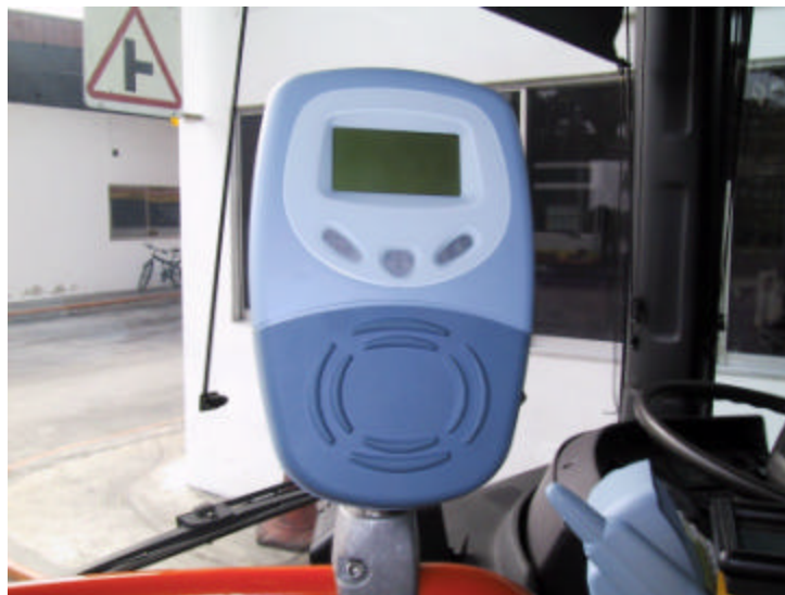
Figure 5. Mockup of an On-Board RFC Reader
