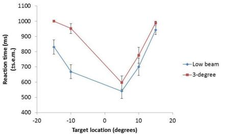
Figure 5. Average reaction times to the onset of targets in the presence of low beam headlights and in the presence of the prototype ADB system evaluated by Skinner and Bullough.<sup>8</sup>
