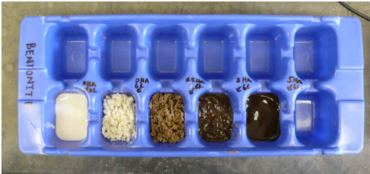
Figure 5.1. Smectite Paste Consistency Prior to Flash Freezing. Note, paste with no lime is liquid and with increasing humic acid content, the paste again reaches liquid consistency.
