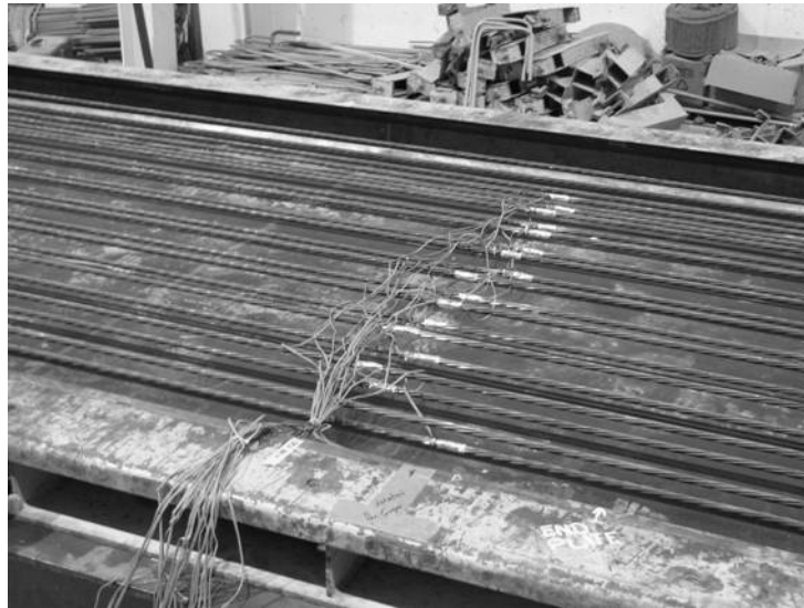
Figure 6.12: Resistive strand gages for measurement of initial prestress force
