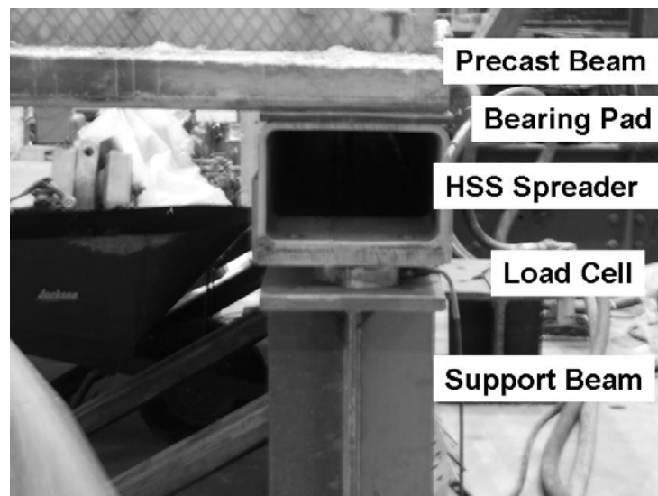
Figure 6.11: Picture of the end reaction with embedded load cell
