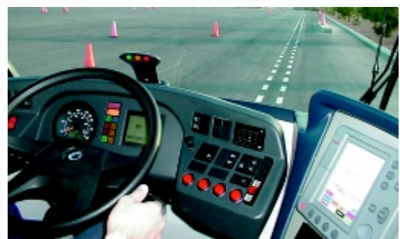
(Top) Bus passengers in Las Vegas are able to board buses more safely and quickly thanks to the precision docking system used on buses owned by the Regional Transportation Commission of Southern Nevada. (Bottom) Video guidance systems assist bus drivers in handling narrow lanes and other hazardous driving conditions. The system above is tracking a paint stripe.
